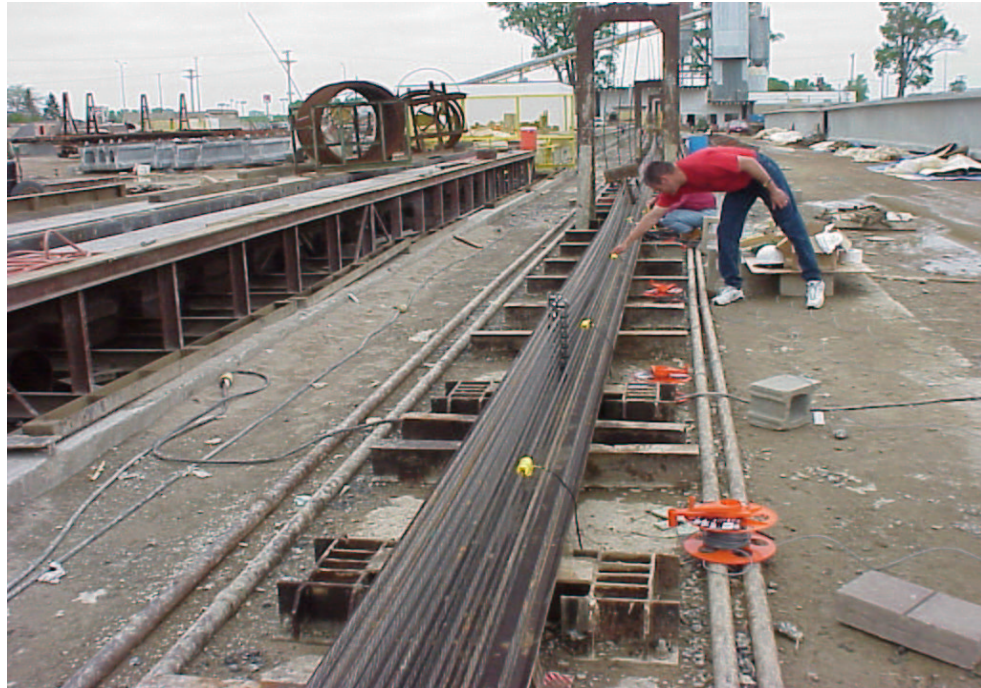
Figure 3. Magnetoelastic sensors installed on a strand
