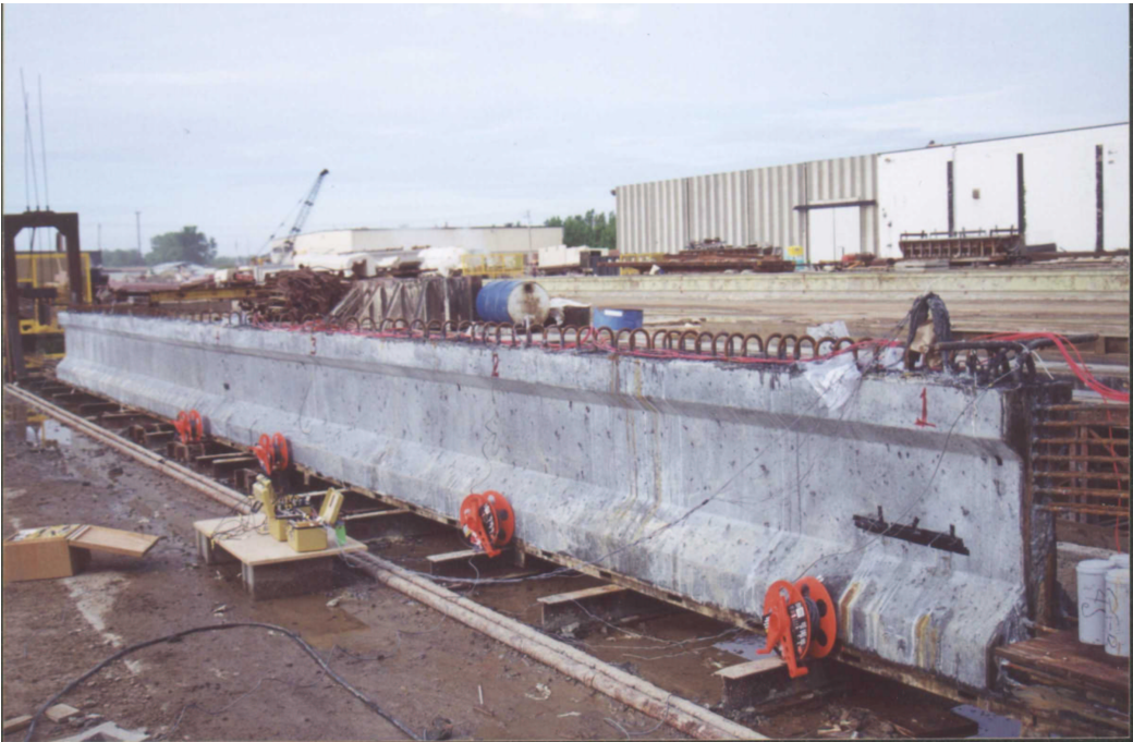
Figure 8. Fabricated pre-tensioned I-beams
