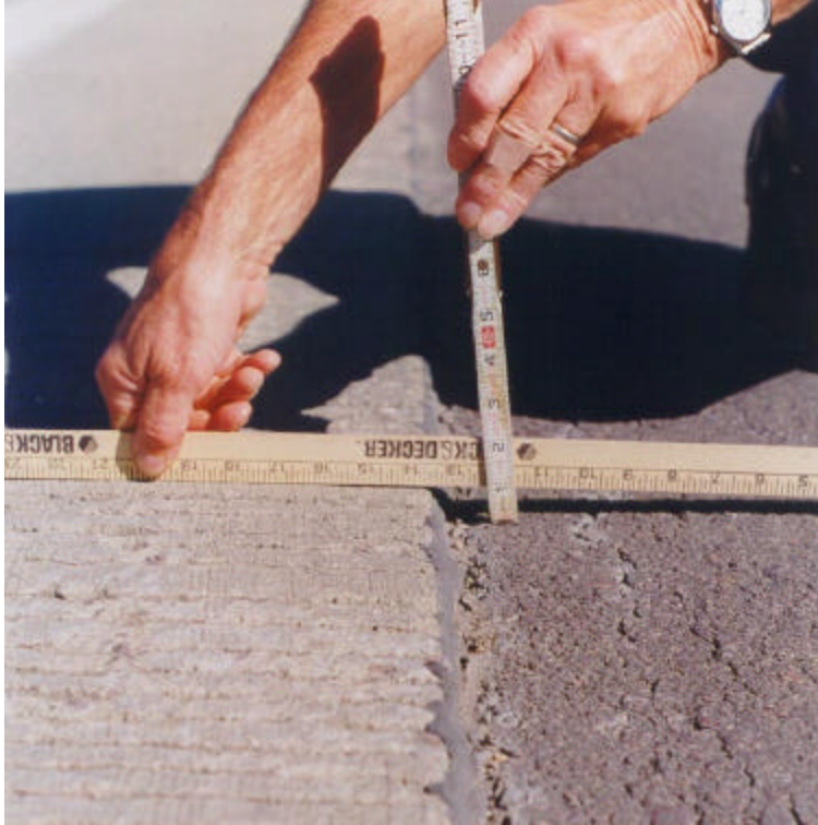
Figure 6. Approximate 1-in shoulder settlement on project 9a (US 12 EB, Bath).
