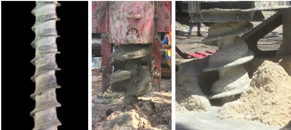
Figure 4.12 (from L to R) soil cuttings adhere to auger stem, soil cuttings sit on auger flights, and an example of a hybrid soil cling mode
