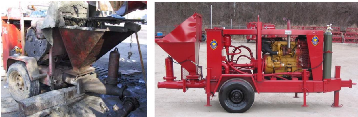
Figure 1.4 Two examples of grout pumps used during auger cast installation; left (Brown et al., 2007) and right (Marinucci & NeSmith, 2017)
