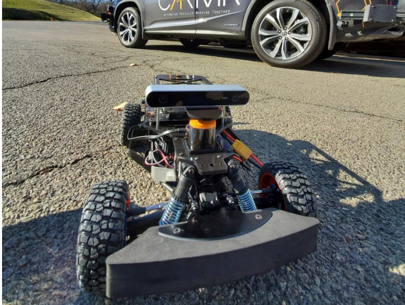
Figure 4. One-tenth scaled-down physical vehicle (CARMA 1Tenth). Source: FHWA
