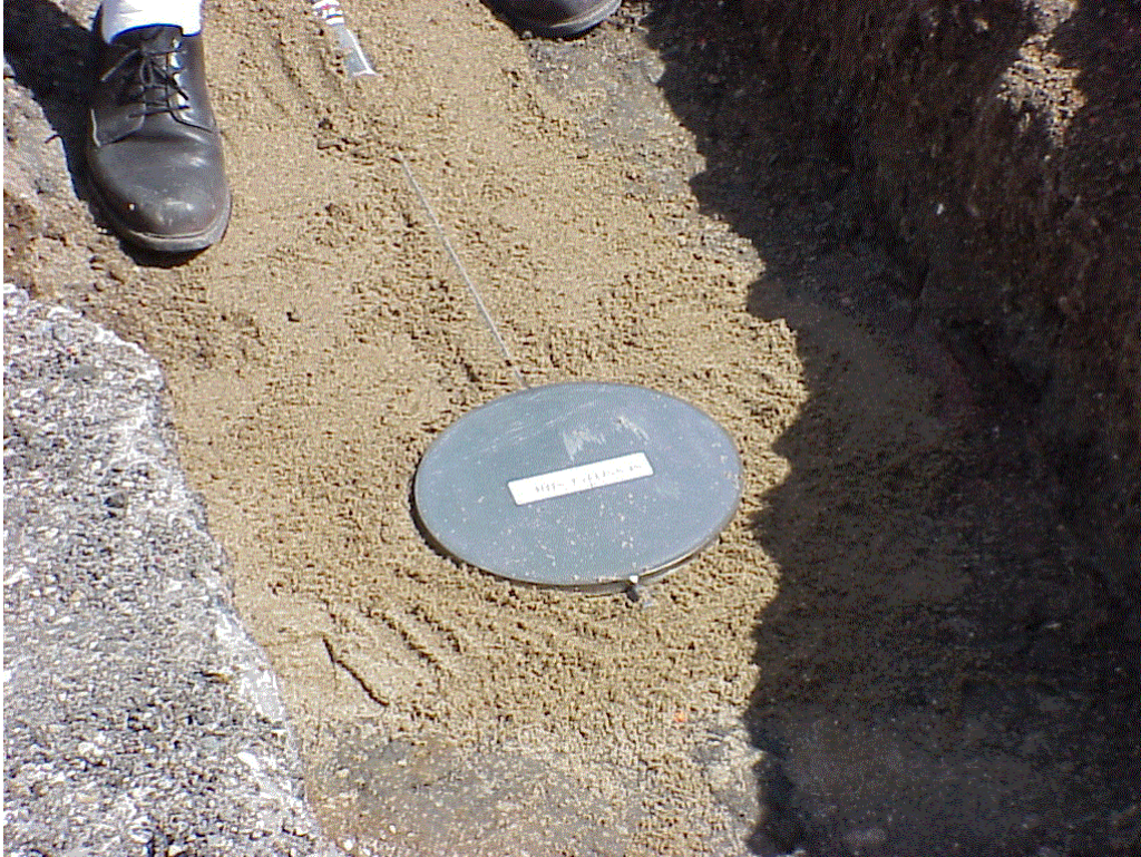
Figure 17: Pressure Cell Installed 4" Into Subgrade
