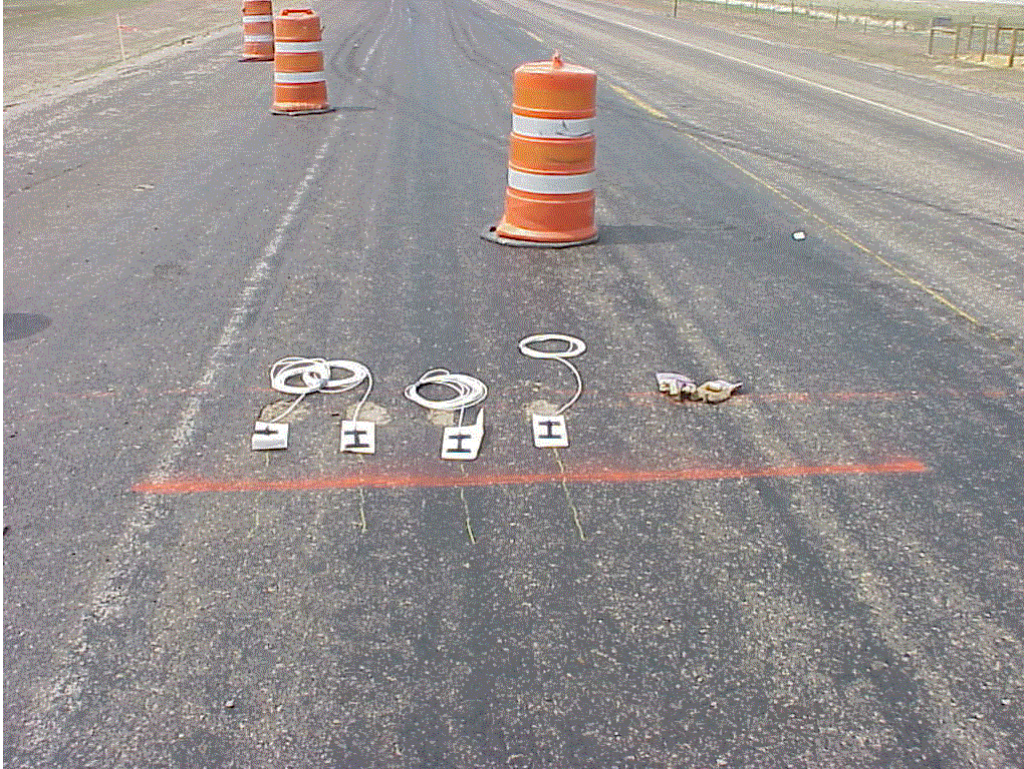
Figure 15: Layout of the Strain Gauges on Top of the Base Course
