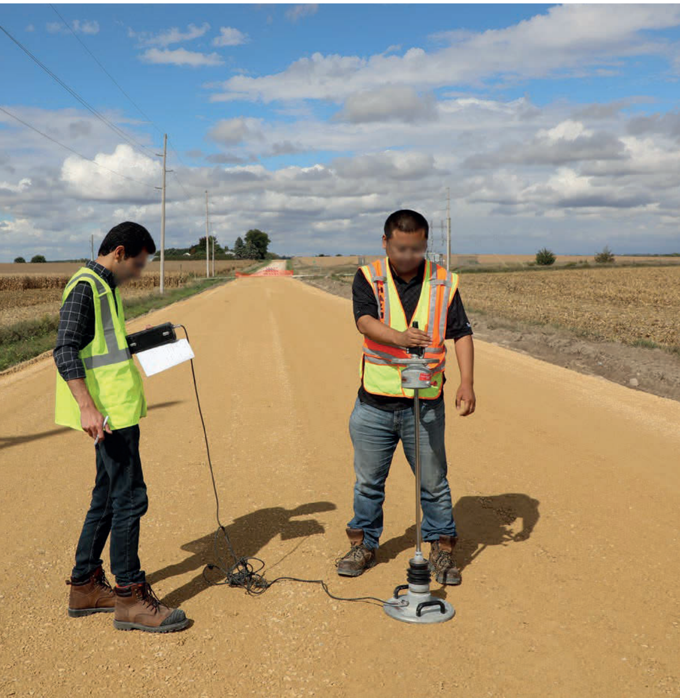
Unpaved road monitoring by field tests (dynamic cone penetrometer test on the subgrade) in Buchanan County. © Araz Hasheminezhad.
