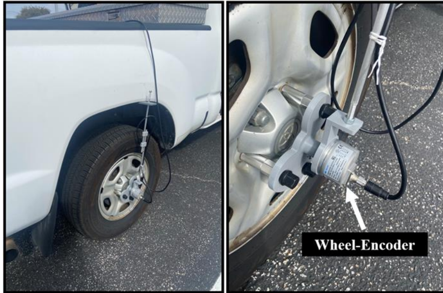
Figure 4.5 Wheel-encoder Installed on rear wheel of test vehicle
