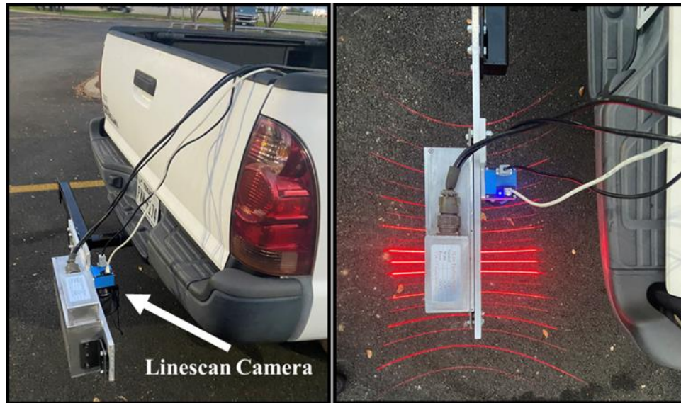
Figure 4.3 Side View and Top View of the Linescan Camera Attached to the Vehicle
