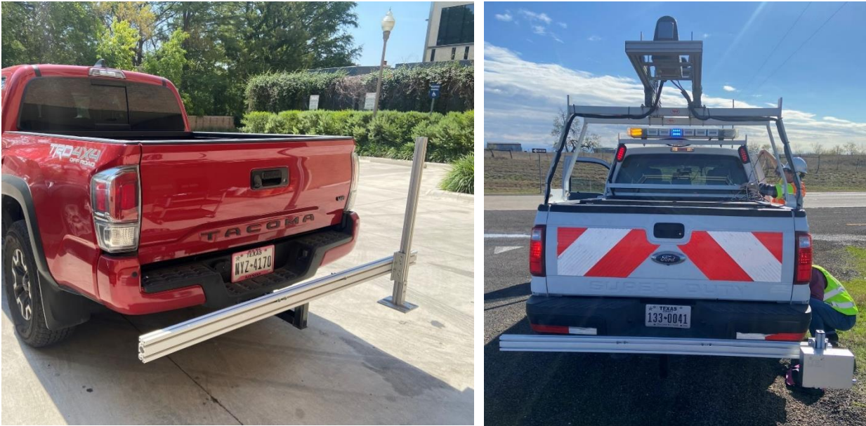
Figure 4.7 (left) UT's test vehicle with mounting system; (right) TxDOT's profiler vehicle with mounting system and product
