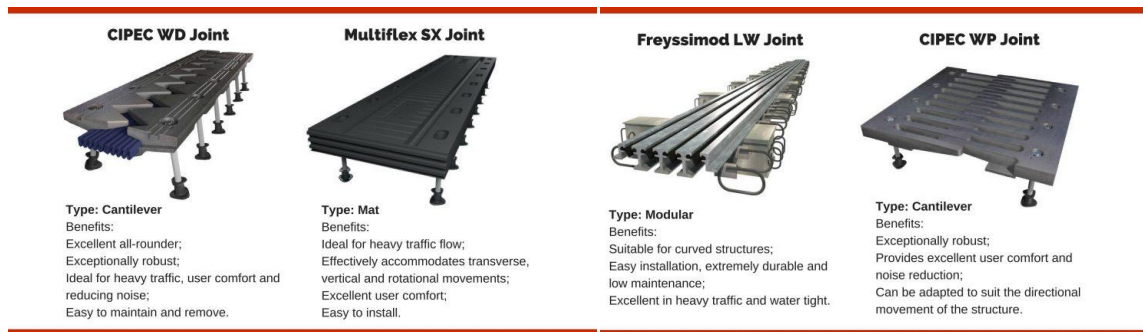
Figure 36 Example of expansion joints
