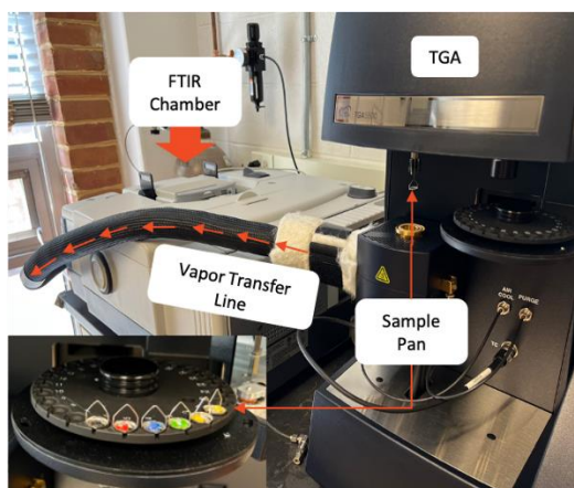
Figure 8. Thermogravimetric Fourier Transform Infrared Analyzer (TGA-FTIR) Instrument Layout
