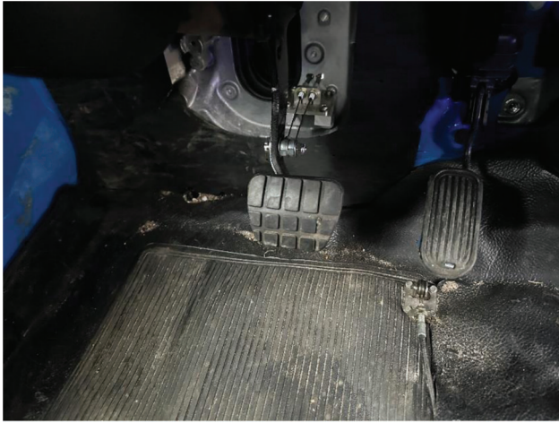
Figure 1.6 Follower truck customized by-wire-control system that controls the brake and gas pedals.
