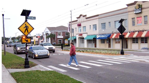
Figure 57. Rectangular rapid-flashing beacons (RRFBs) mounted on posts, St. Petersburg, FL (Image: Michael Frederick/pedbikeimages.org [open source])
