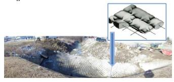
Design C: Low-head weir downstream the culvert
