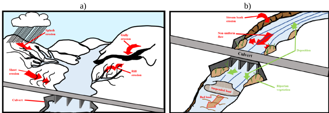
Figure 1. End-to-end culvert sedimentation processes: a) soil detachment (sediment production and overland transport) in the culvert drainage area; b) in-stream sediment transport to culvert vicinity and deposition processes in the vicinity of the culvert (Muste and Xu, 2017).
