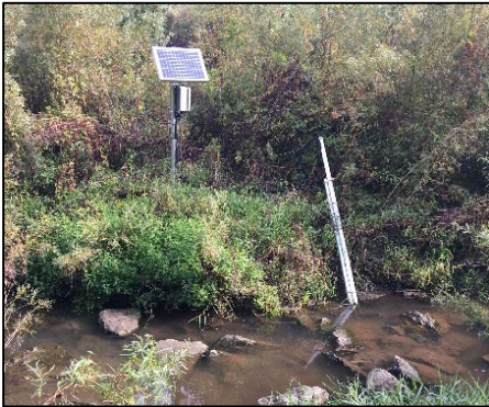
Figure 17. Deployment of continuous monitoring sensors for quantification of the hydrologic/hydraulic and morphological variables at the study sites: a) Hwy 1 on Clear Creek in Iowa City (FHWA #31711); b) Mormon Trek Blvd. on Clear Creek in Iowa City (FHWA #364790)
