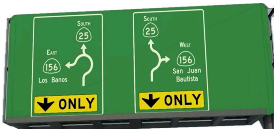
Figure 12: Sign used on entry lanes ahead of a turbo roundabout (Image source: Caltrans, 2023)
