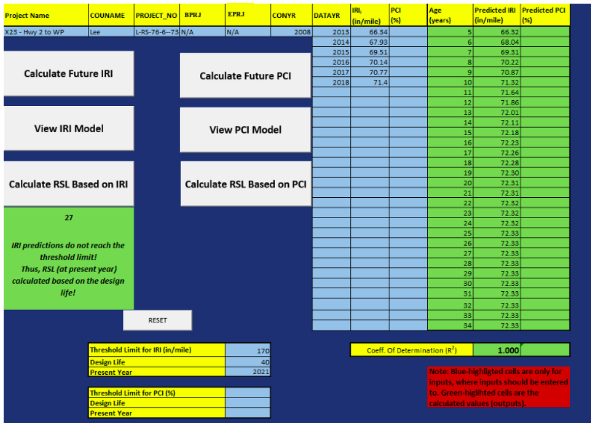
Figure 72. Threshold limit for IRI (170 in./mi), design life (40 years), and present year (2021): AC (statistics-based model)
