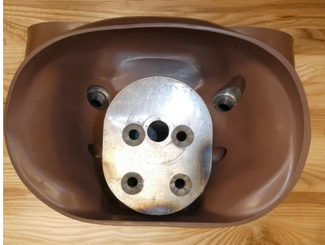
Figure 5: Pelvis to MTS Adapter Mounted on a Pelvis (Top View)
