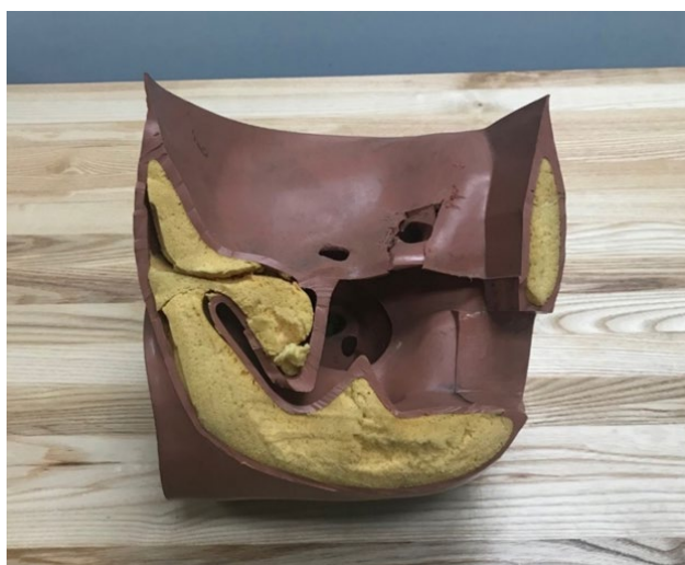
Figure 1: Pelvis Foam and Rubber Shell Cross-Section
