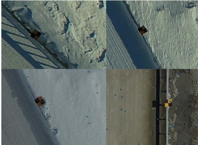
Figure 3.5. A collage of pictures collected from the RPAS of a GCP on the guardrail. From upper left clockwise: February 4th, February 11th, March 3rd, and April 29th. Among the four pictures, only the GCPs at the bottom of the figure were automatically detected by Metashape.
