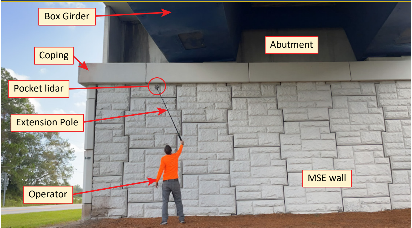
Figure 2. Illustration. Data collection procedure with a PL unit on an extension pole.
