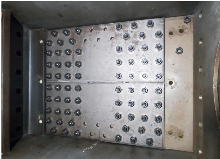
Figure 5.11: Specimen A: spliced section after fracture due to uneven distribution of liquid Nitrogen (photo taken inside the specimen)
