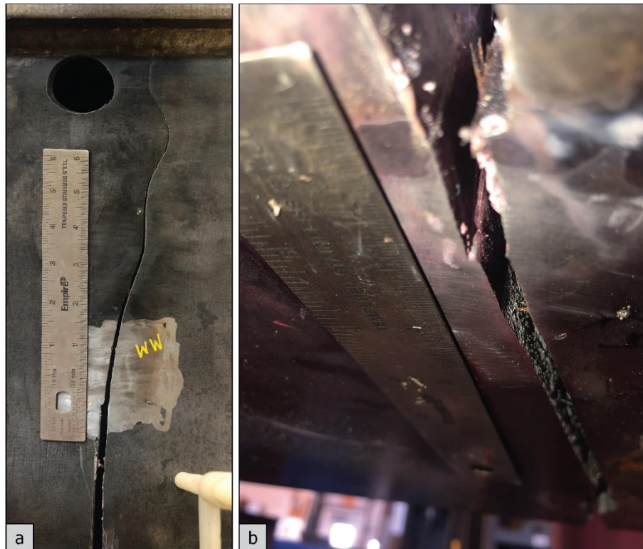
Figure B.22: Fracture obtained in the West web (a) and bottom flange (b)
