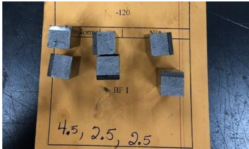
Figure 4.17: CVN specimens tested at -120 °F (bottom flange plate)
