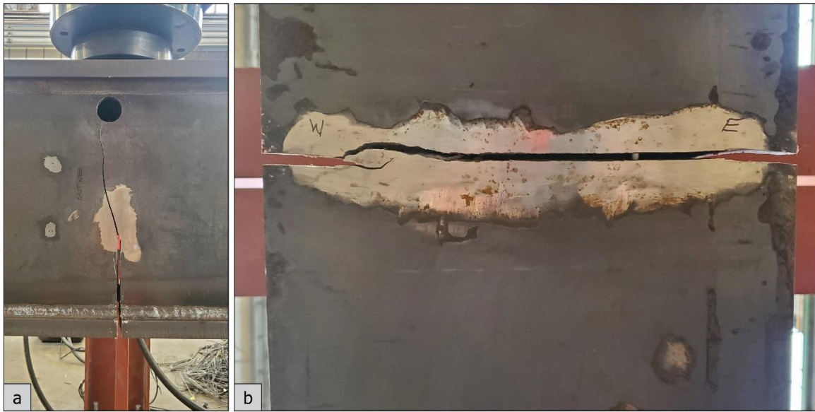
Figure B.30: (a) East web and (b) bottom flange cracks produced in PS2A fracture test.
