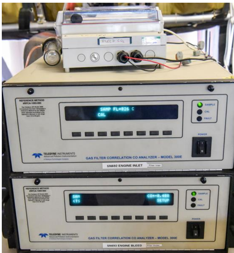
Figure 43. NDIR analyzers for carbon dioxide and carbon monoxide
