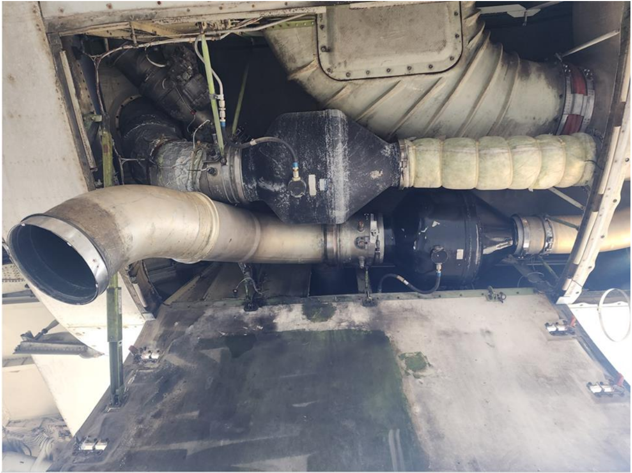
Figure D-13. Pack exit duct rotated down and reinstalled to coalescer without ground port - upward view
