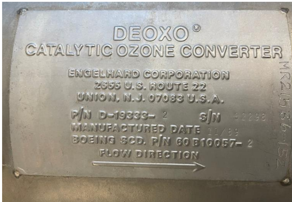
Figure 5. Name plate on #1 ozone converter, converted to a VOC/ozone converter
