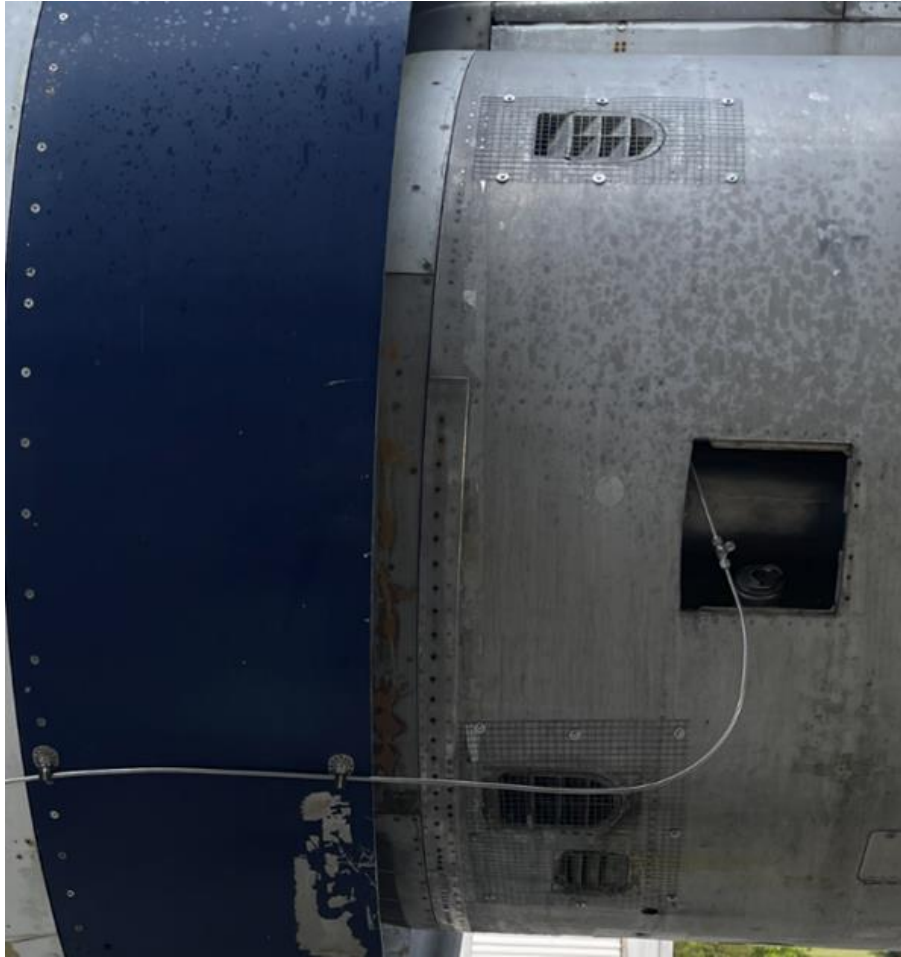
Figure 26. Securing stainless injection line to number 3 engine
