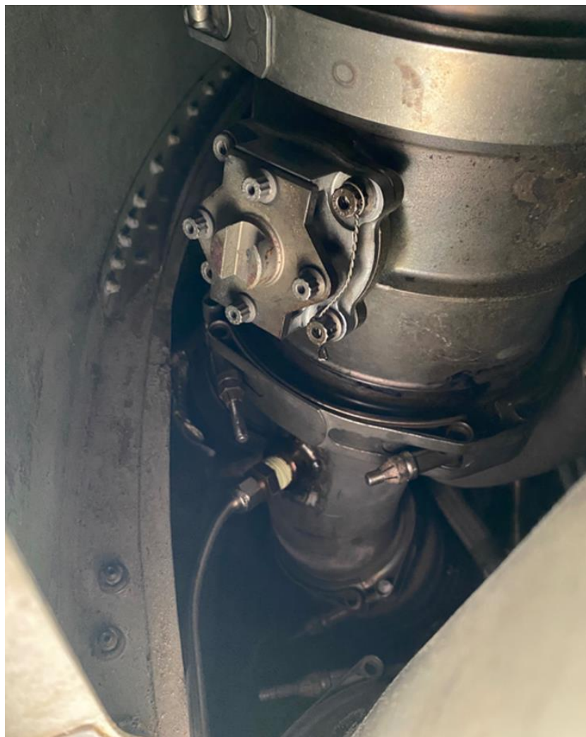
Figure 27. Contaminant injection port on number 3 engine bleed duct
