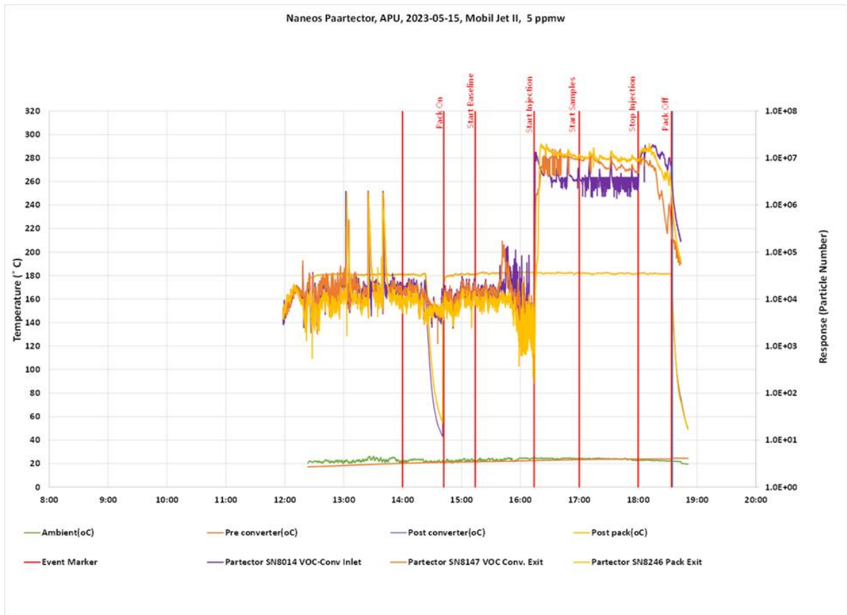
Figure 64. Total ultrafine particle concentration, Naneos Partector, May 15, 2023, APU, Mobil Jet Oil II, 5 ppmm (nominal)
