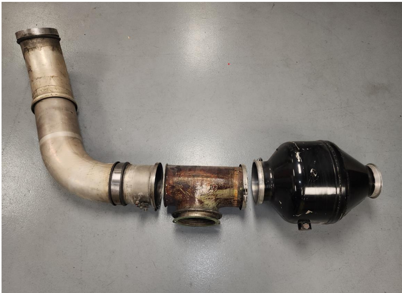
Figure D-11. Aircraft environmental control system duct modification Ground air conditioning port and coalescer housing removed
