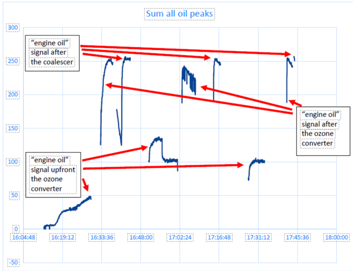
Figure 112. Measurement of bleed air from APU with AT upstream and downstream of VOC/ozone converter and at pack exit during injection of Mobil Jet Oil II, 5 ppm
