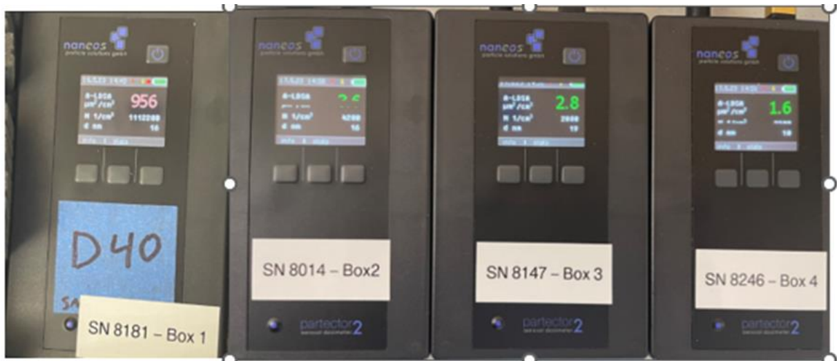
Figure 39. Naneos Partector II UFP detectors
