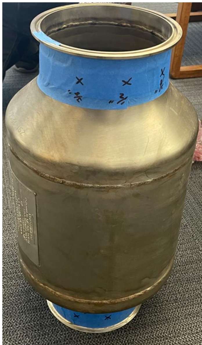
Figure 7. #1 ozone converter marked for bung attachments
