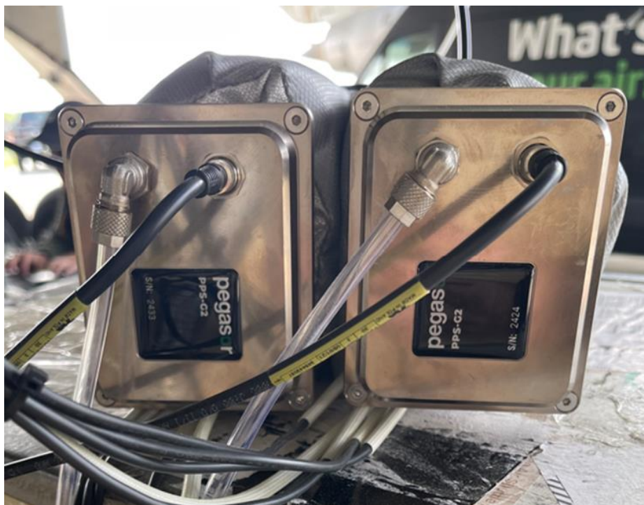
Figure 36. Pegasor heated UFP analyzers
