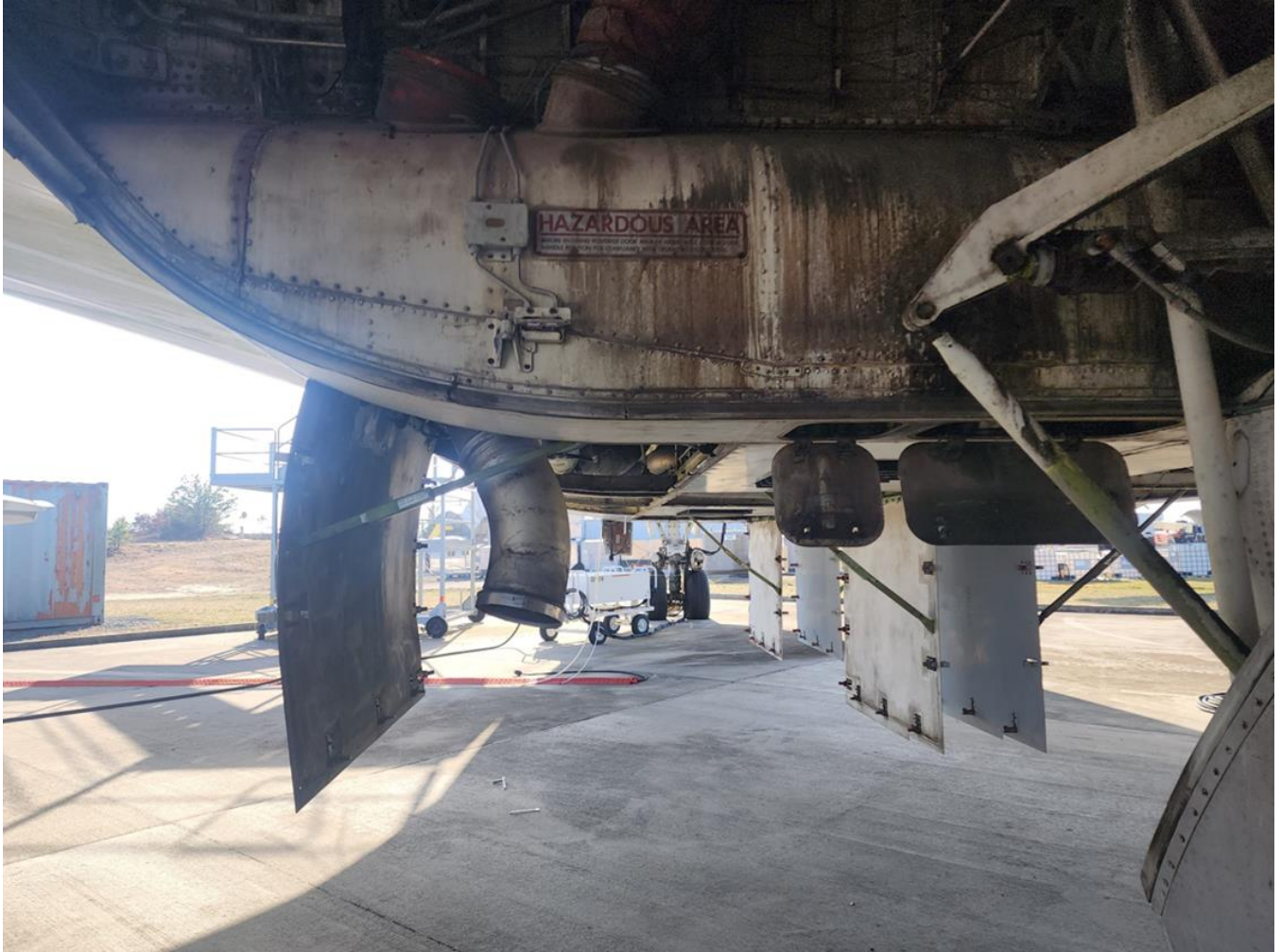
Figure D-15. Duct rotated down and reinstalled to coalescer without ground port Looking forward towards aircraft nose from aft wheel well
