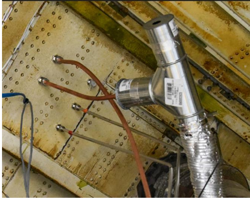
Figure 33. Sample adapters penetrating cabin bulkhead
