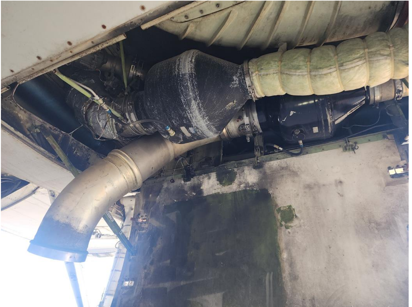
Figure D-14. Pack exit duct rotated down and reinstalled to coalescer without ground port - side view
