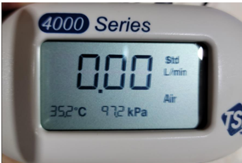
Figure 52. TSI Model 4000 flowmeter transfer standard for mass flow controllers
