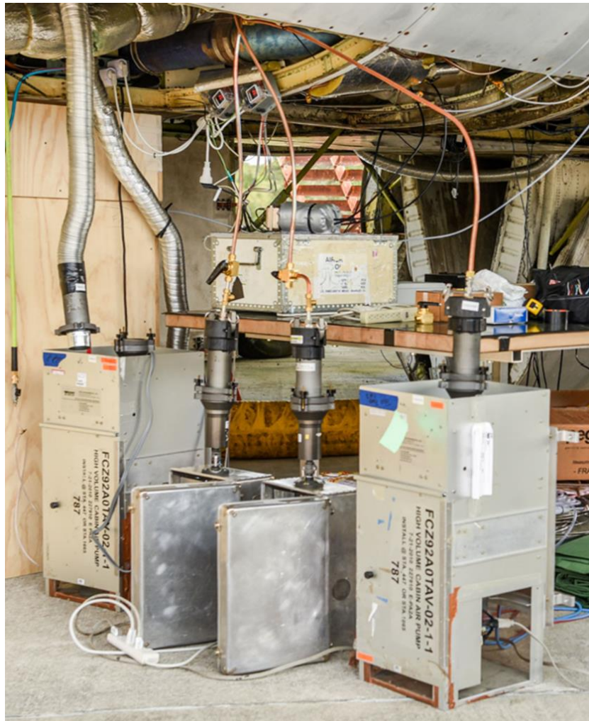
Figure 53. Tisch™ 102 mm quartz filter sample assembly
