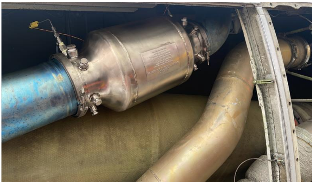
Figure 8. VOC/ozone converter reinstalled for bleed air test
