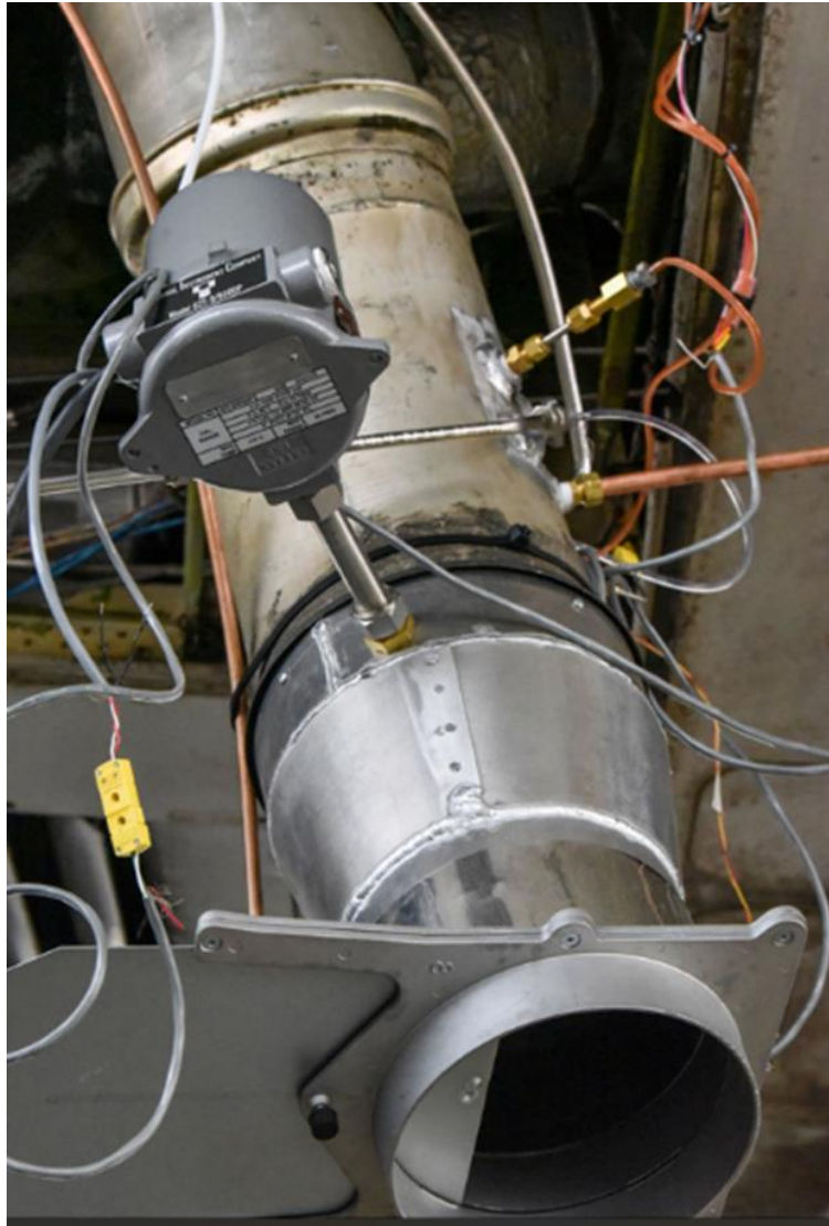
Figure 29. Total bleed air flow measurement and sample lines at pack exit
