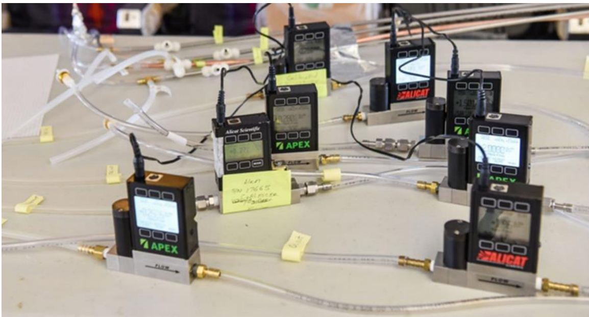
Figure 51. Mass flow controllers with DNPH and Tenax thermal desorption tubes
