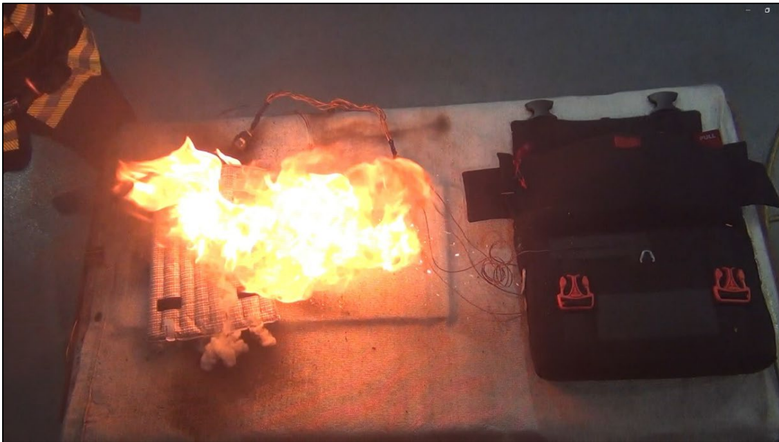
Figure 8. Manufacturer A – power bank catches fire outside of bag
