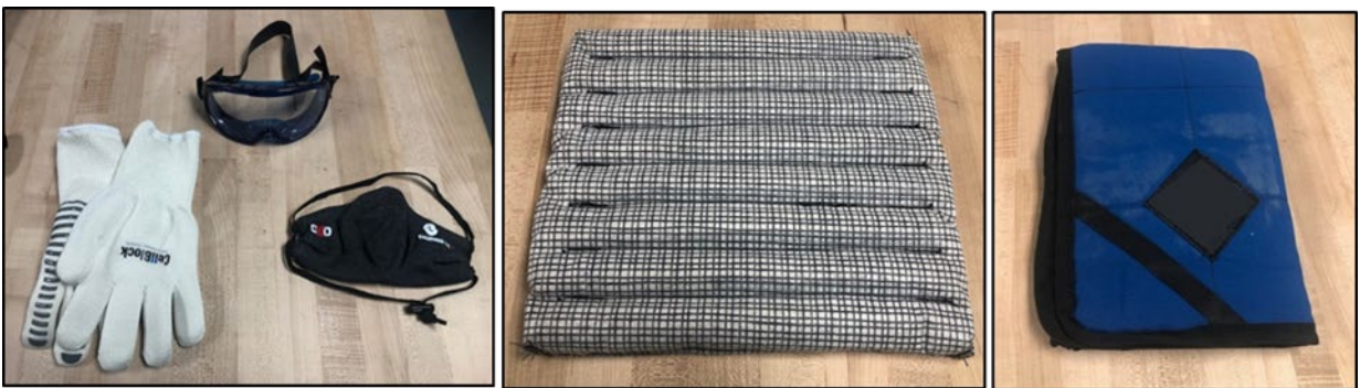
Figure 5. PPE (left), fire suppression pad (middle), and folded up fire blanket (right)
