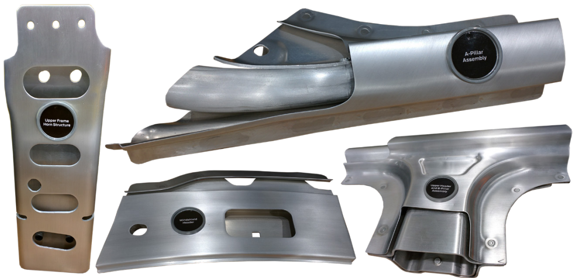
Figure 2: Photographs of aluminum components used in the 2015 Ford F-150
