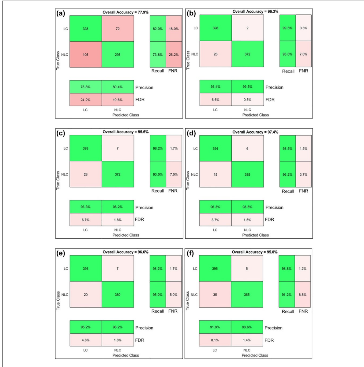
Figure 14 Confusion matrices of the best performing lane change detection models using ResNet-18 for six data categories: (a) Category 1 (vehicle kinematics); (b) Category 2 (machine vision); (c) Category 3 (vehicle kinematics + machine vision); (d) Category 4 (vehicle kinematics + roadway geometry + machine vision); (e) Category 5 (vehicle kinematics + machine vision + driver demographics); and (f) Category 6 (vehicle kinematics + roadway geometry + machine vision + driver demographics).
