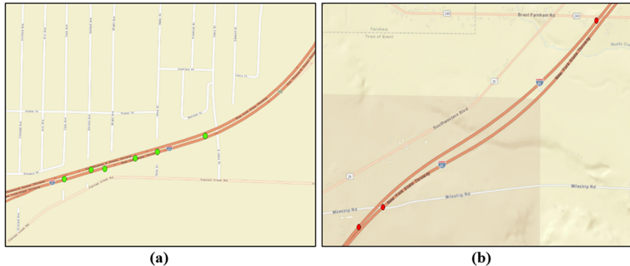
Figure 21 Identification of lane-change events occurring in various freeway facilities: (a) lane-change events in a freeway weaving segment (I-90, New York) and (b) lane-change events in a basic freeway segment (I-90, New York).
