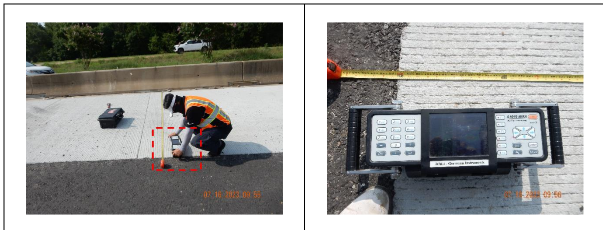
Figure 75 MIRA scanning performed in a selected slab.
