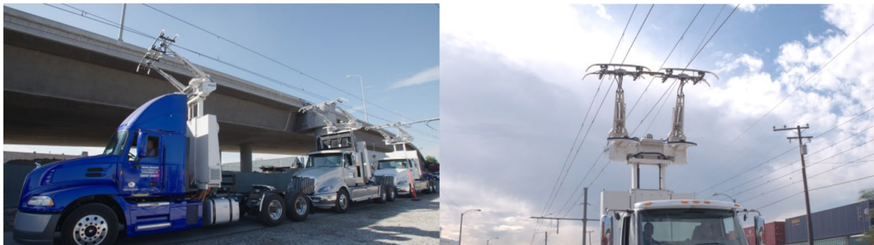
Figure 18 One-mile, zero-emission eHighway demonstration in Carson, California conducted by Siemens. Source: https://www.greencarcongress.com/2017/11/20171109-siemens.html
