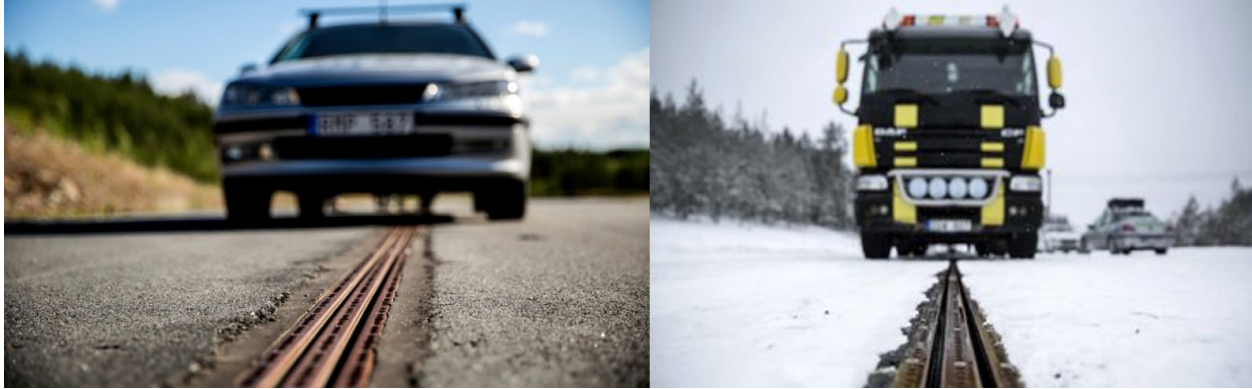
Figure 19 Electrified road for charging in Stockholm, Sweden. Source: https://www.theguardian.com/environment/2018/apr/12/worlds-first-electrified-road-for-charging-vehicles-opens-in-sweden
