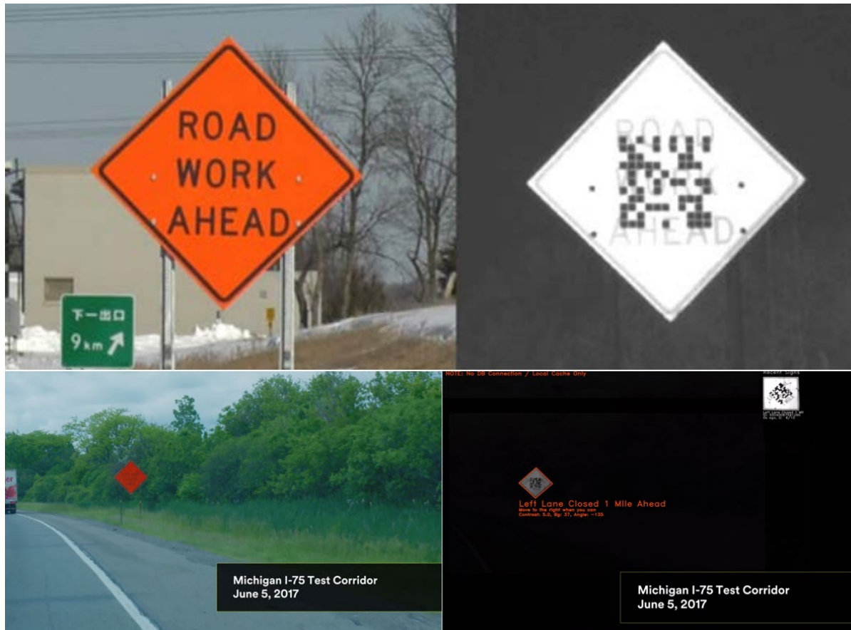
Figure 16 Machine vision to recognize traffic signs using barcode by 3M. Source: “Invisible” 2D Bar Code to Enable Machine Readability of Road Signs – Material and Software Solutions - 3M Transportation Safety Division
