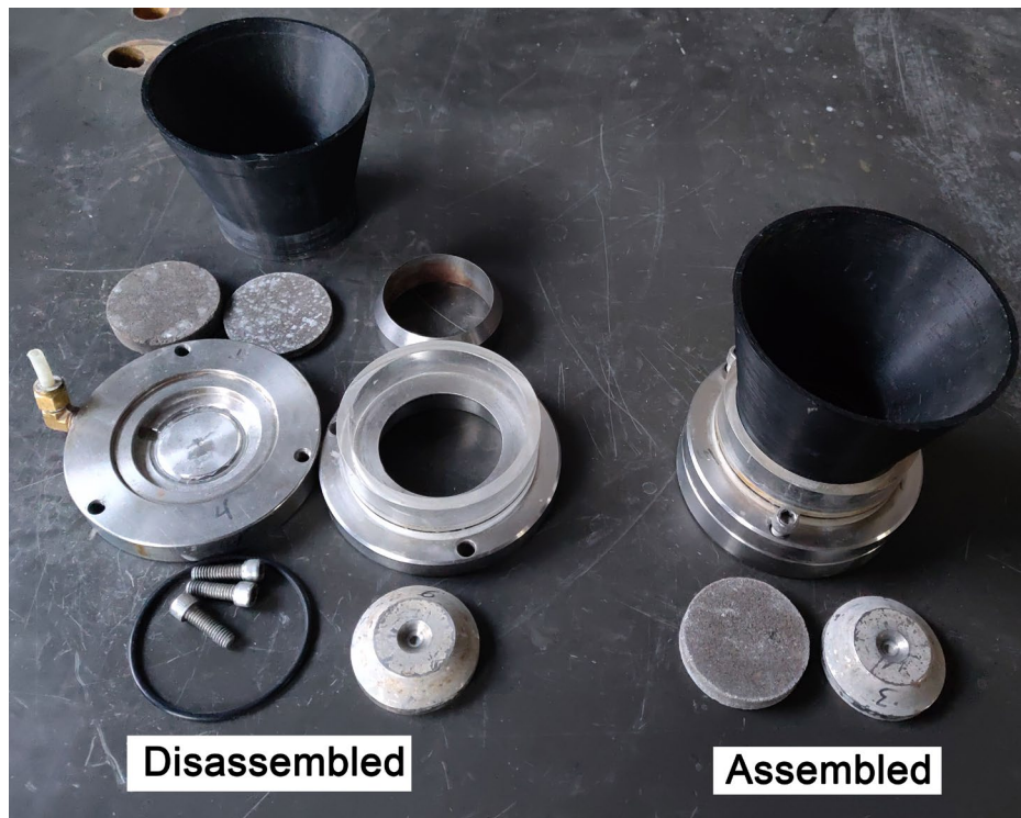
Figure 3.6 Figure Showing the Consolidation Cell Assembly and the Funnel Apparatus
