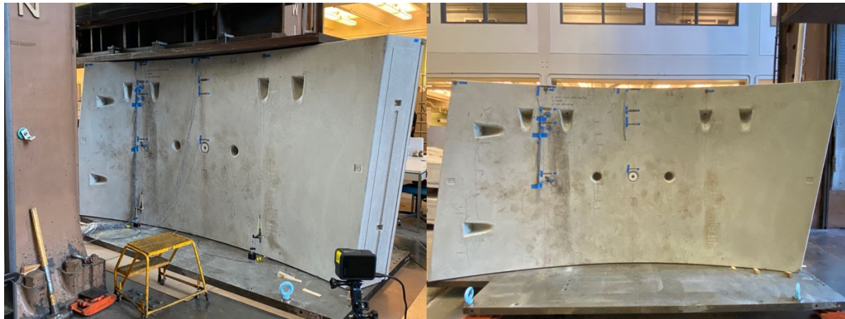
Figure B2-1: Intrados image of segment before (left) and after (right) testing.
