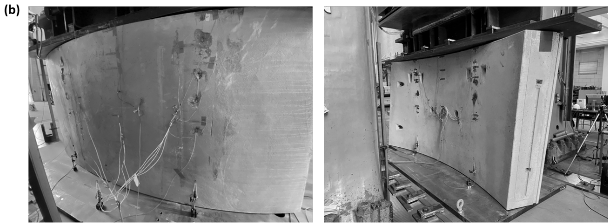
Figure 2-8. (a) Segment instrumentation layout for thrust jack loading including radial and tangential strain gages on the segment intrados and extrados, and (b) photos of radial and tangential strain gages and displacement transducers on the segment intrados and extrados.
