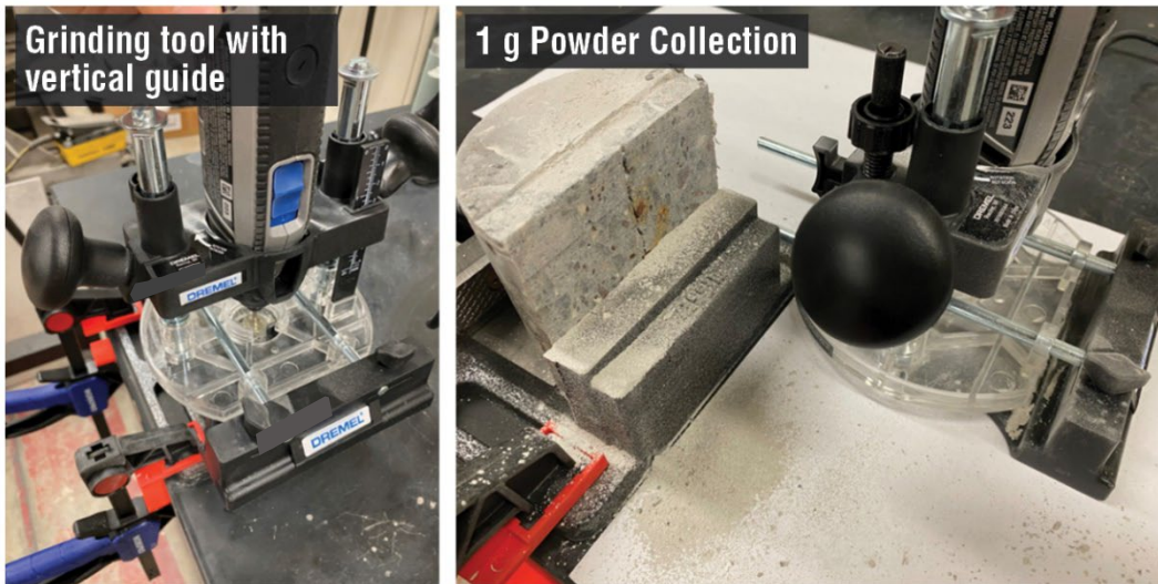
Figure 4-8. Grinding procedure to prepare sample for IC chloride analysis.
