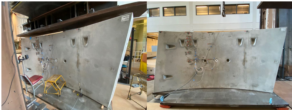
Figure B4-1: Intrados image of segment before (left) and after (right) testing.
