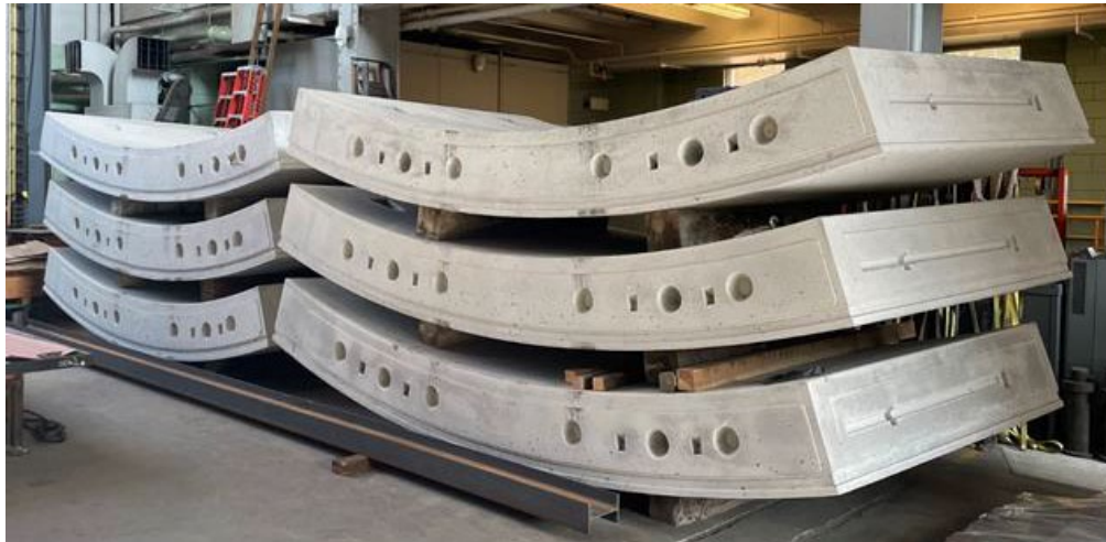
Figure 2-3. Batch of precast tunnel lining segments used for thrust jack testing. Segment dimensions are 4.06 m (13.5 ft) long, 2.0 m (6.5 ft) wide and 457 mm (18 inches) thick.
