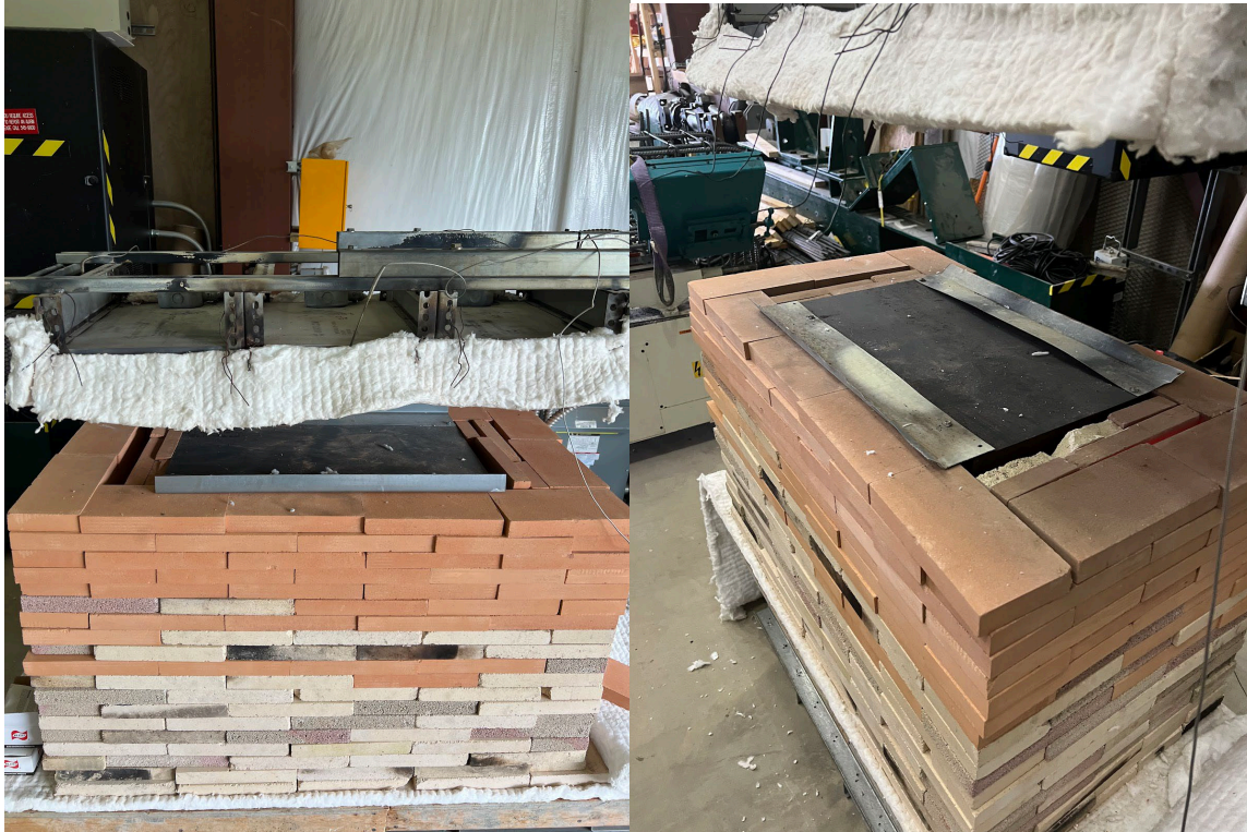
Figure 3-3: Condition of the top flange and decking before (left) and after (right) testing
