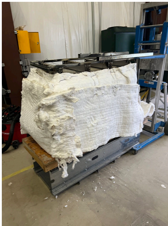
Figure 2-5: Ceramic fiber insulation wrapped around the firebricks and heater setup
