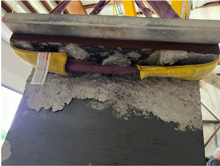
Figure 3-9: Fireproofing chipped off the top flange of the scenario 2 beam
