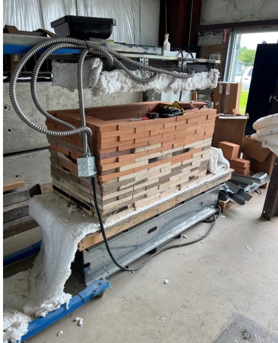
Figure 2-4: Firebricks, heaters, and insulation setup
