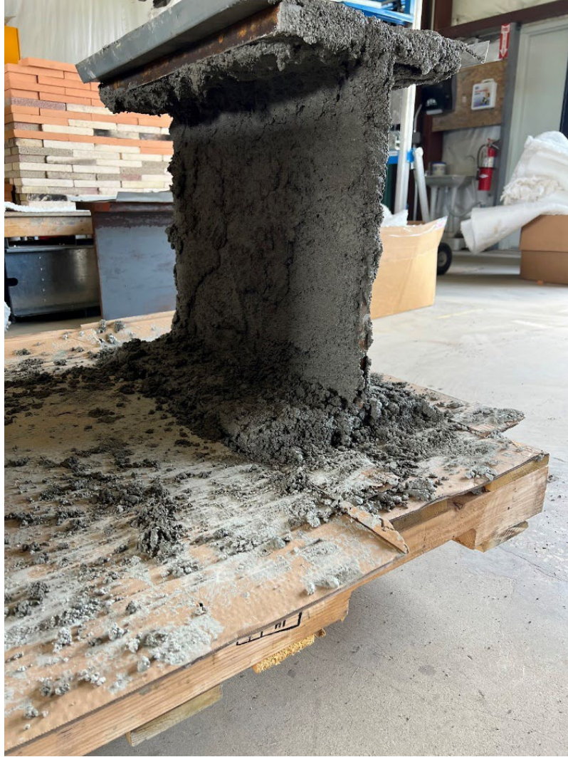
Figure 2-15: Fully fireproofed scenario 1 beam
