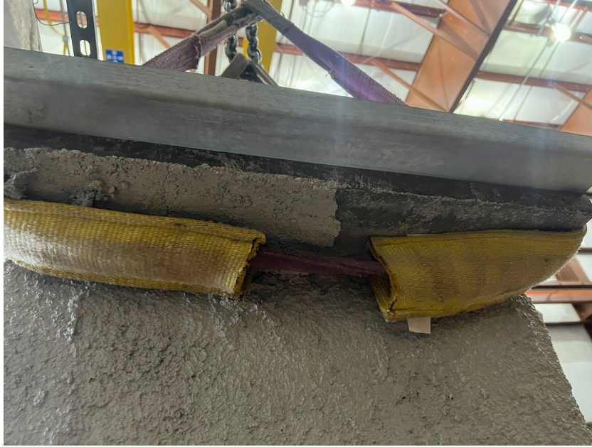
Figure 3-14: Fireproofing damage on the underside of the top flange for scenario 3.
