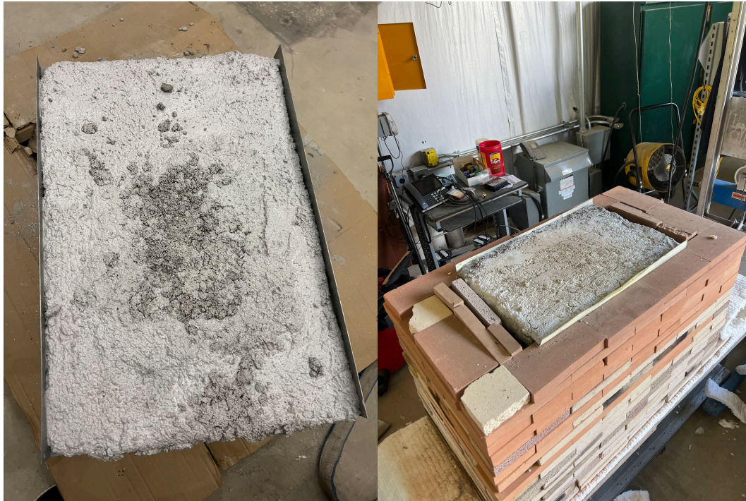
Figure 3-7: Fireproofing on the scenario 1 beam before and after testing
