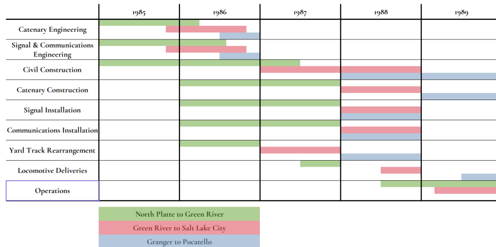
Figure 4. Planned Construction Timeline for the UP Electrification
