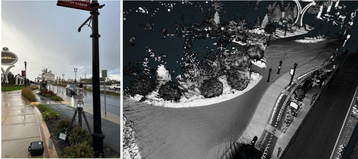
Figure 2.1: LiDAR scanning set up and corresponding cloud point data (Broadway at Horizon Way Street.)
