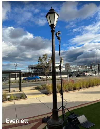
Figure 2.10: LiDAR scanning scene for infrastructure and trajectories (Somerville Avenue and Stone Avenue, Somerville, MA)
