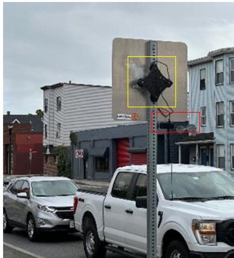
Figure 2.9: Configuration of the 360° video camera (with battery and the camera magnetically mounted on the sign post as shown in the yellow and red boxes)
