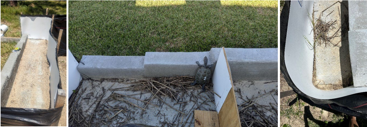
Figure 13. Photo. Runway trial. Left: Polywall ® placed around entire inside perimeter of runway trial. Middle: Divider separating 6” and 8” height curbs from 10” and 12” curbs. Right: Polywall ® curved at corners to replicate directional fencing.
