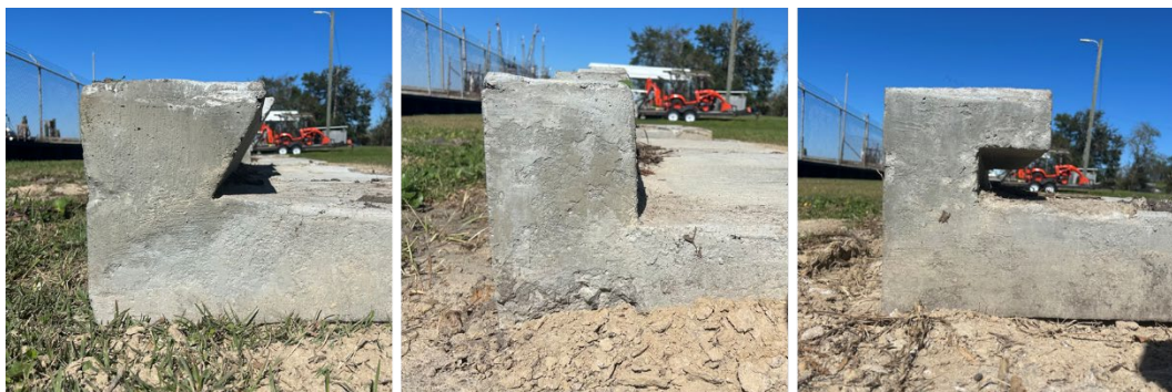
Figure 3. Photo. Curb cut sections. Cut section images of all three curb designs at the 6” height for reference to table in Figure 2.
