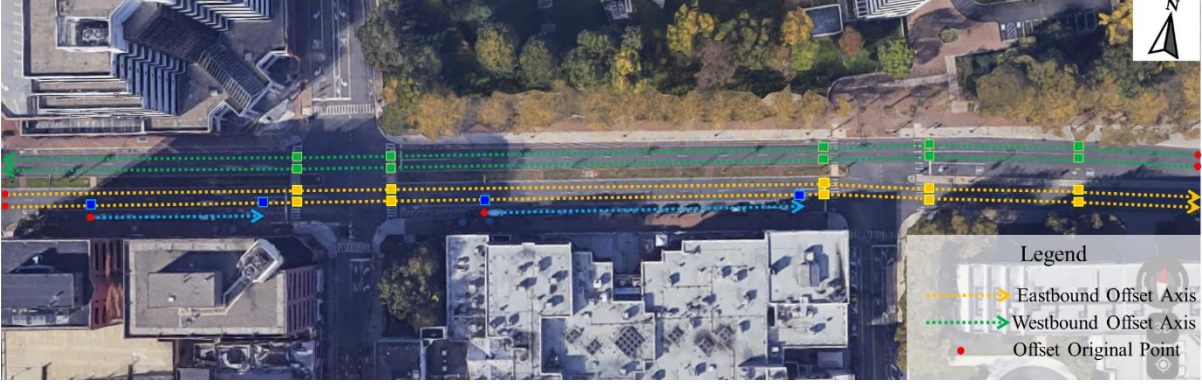
Figure 94. Schematic Diagram of Lane-based Offset Coordinate System for Through Movements (Red Dots: Network Entry points, Arrows: Network Ending Points, Direction of Traffic, Yellow Squares: Waypoints of Major Road Geometry Changes, Yellow: Eastbound (EB), Green: Westbound (WB), Blue: Parking)
