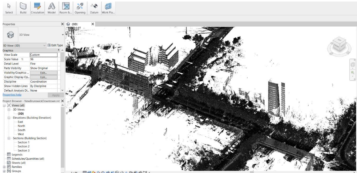
Figure 41. Autodesk Recap Format Point Cloud Loaded in Autodesk Revit
