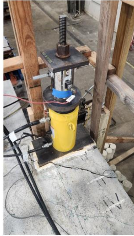
(c) Shear crack from top view
