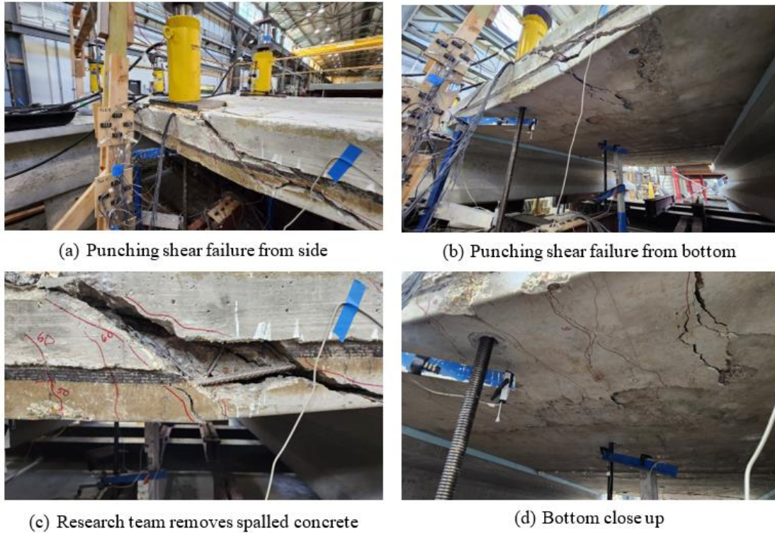
Figure 4-40: Test 8 – Electro-Welded Panel Pair Positive Moment Long Span – Punching Shear at Ultimate Load
