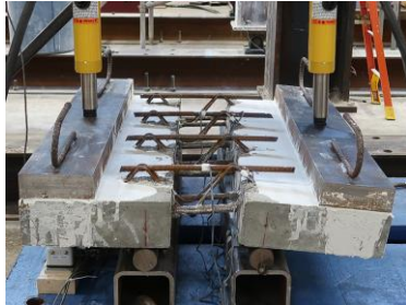
(a) After failure
