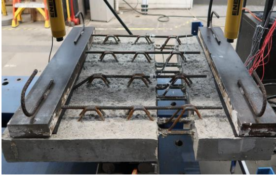
(a) Before testing (the trusses do not extend far into the right-side panel of the specimen)
