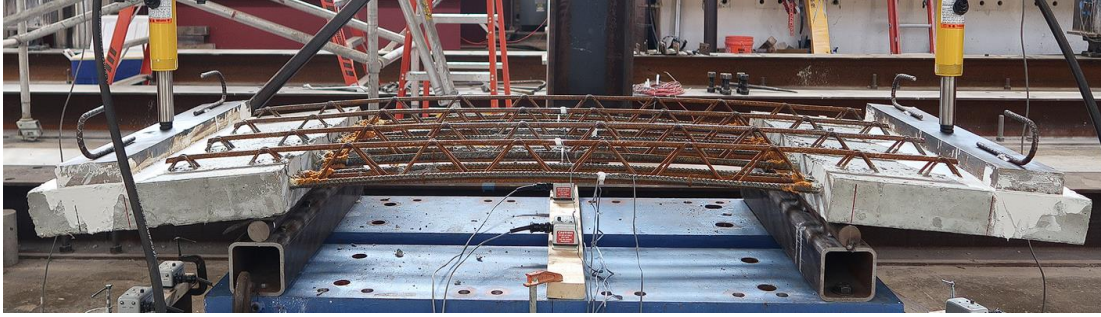
Figure 3-24 Specimen II-E-U49-#4 exhibits large deflections without buckling of trusses
