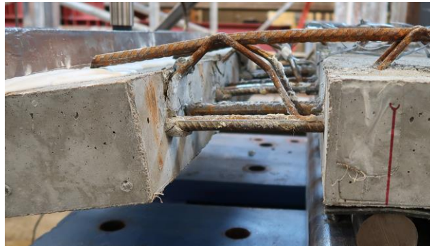
Figure 3-27 Web members buckle during shear testing of Specimen III-E-U6-SW
