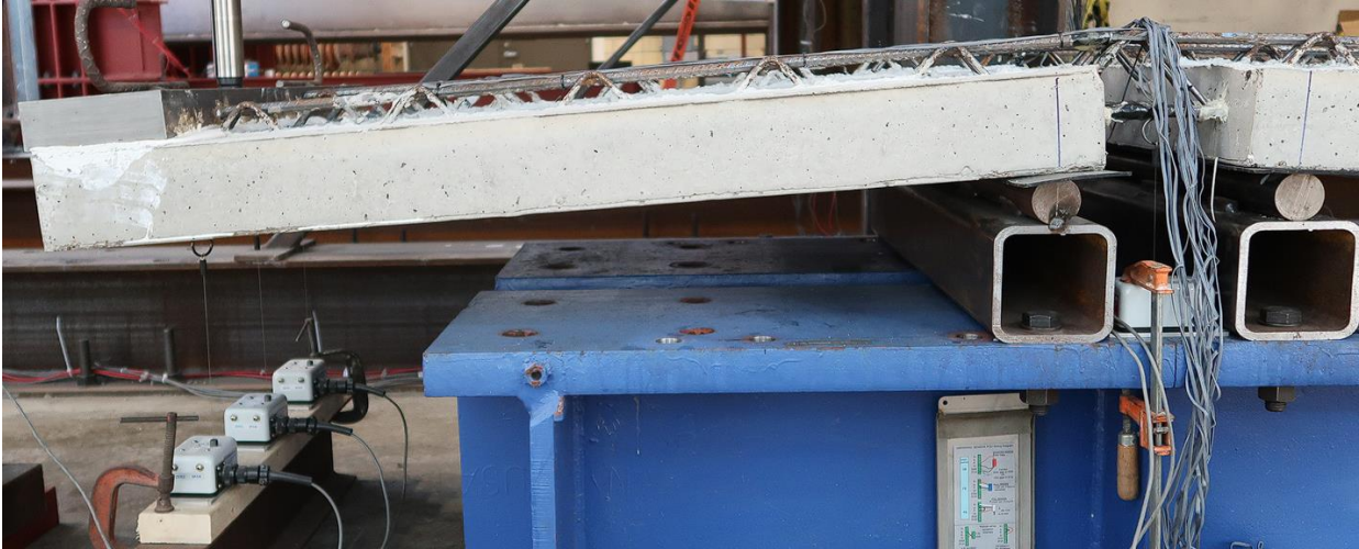
Figure 3-21 Extreme deflection prompts the end of a load test
