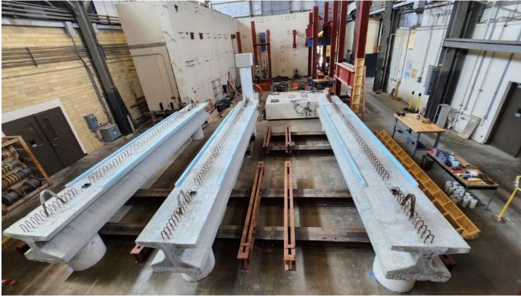
Figure 4-12: Supports and Tx28-girders
