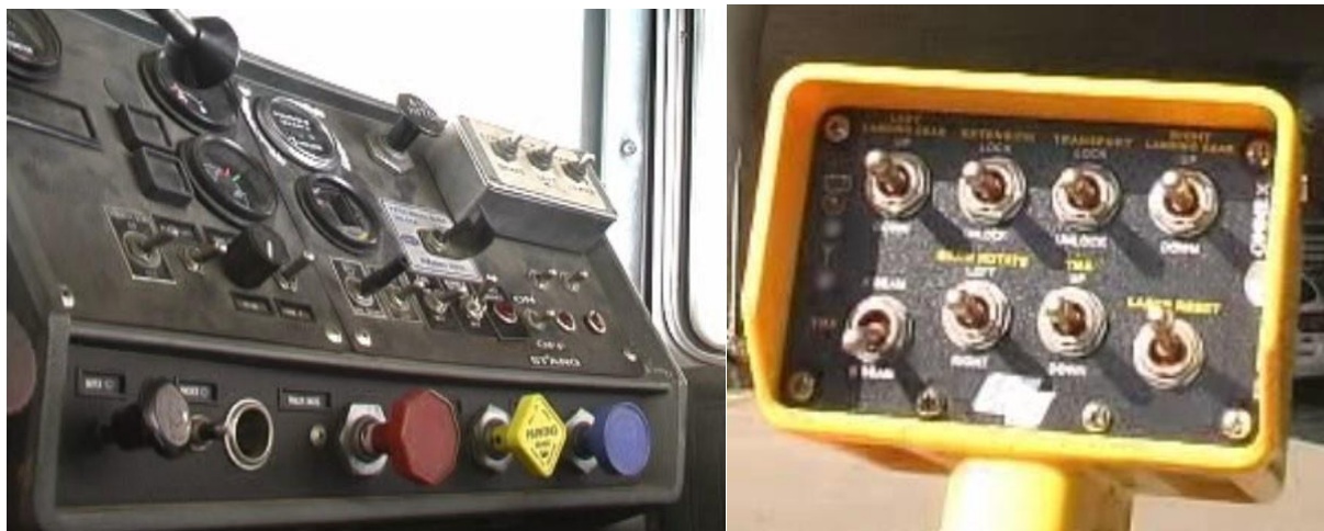
Figure A.4: Balsi Beam inside and remote-control consoles used to deploy/stow.
