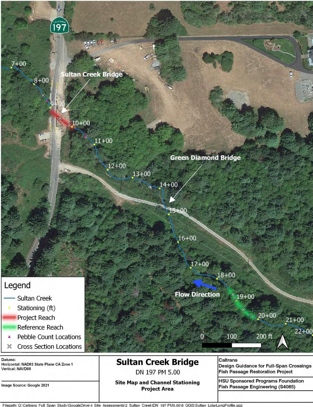
FIGURE 2-2. PROJECT AREA MAP FOR SULTAN CREEK SHOWING CHANNEL ALIGNMENT, PROJECT AREA, REFERENCE REACH, AND CROSS SECTION AND PEBBLE COUNT LOCATIONS.
