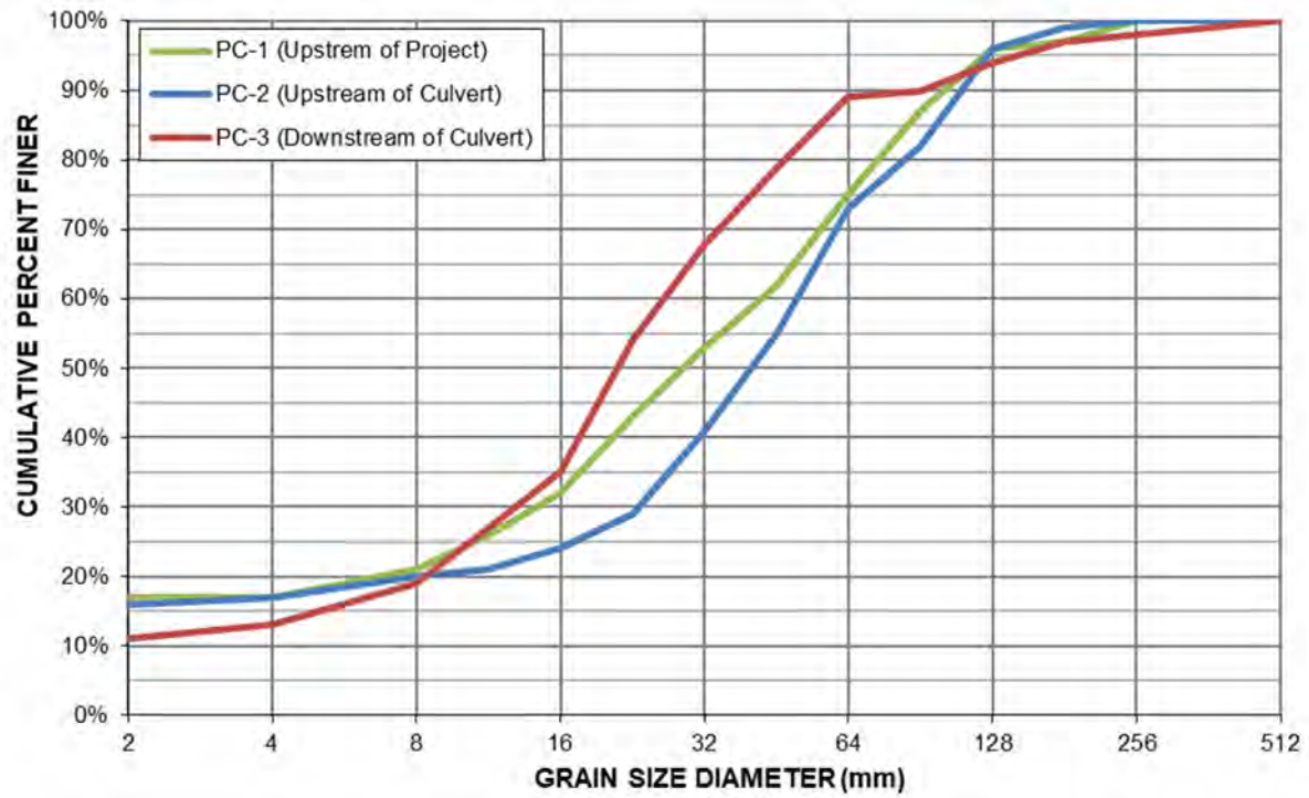
FIGURE 1-6. STREAMBED GRADATION BASED ON SURFACE PEBBLE COUNTS TAKEN DOWNSTREAM AND UPSTREAM OF THE CROSSING AND UPSTREAM OF THE LARGE WOOD JAM.
