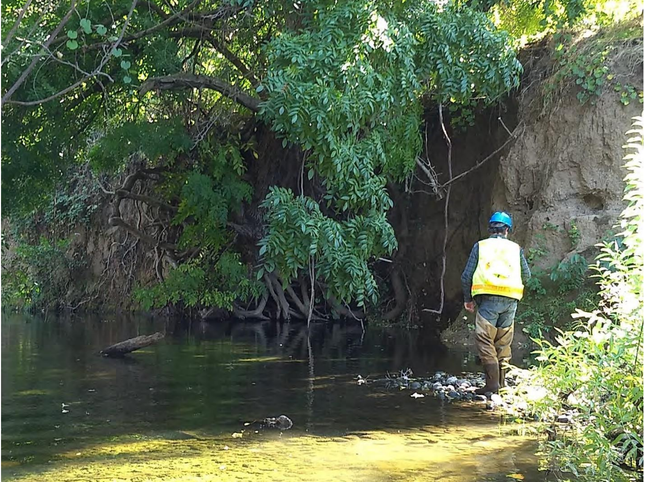
Figure 5. Craig Creek downstream channel showing extreme incision that is not related to the crossing but could influence conditions through the crossing. Photo taken October 4, 2019.
