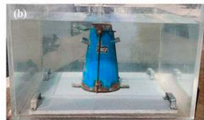
Mock-up test assessing UWC flowability: (a) Slump flow test in the air and (b) Underwater slump flow test.
