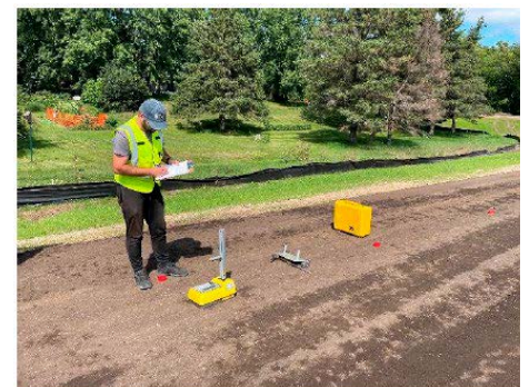
In-place density and moisture content test by nuclear density gauge (NDG) in Dane County (left) and St. Croix County (right)
