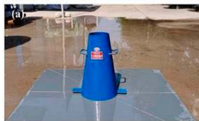
Mock-up test assessing UWC flowability: (a) Slump flow test in the air and (b) Underwater slump flow test.
