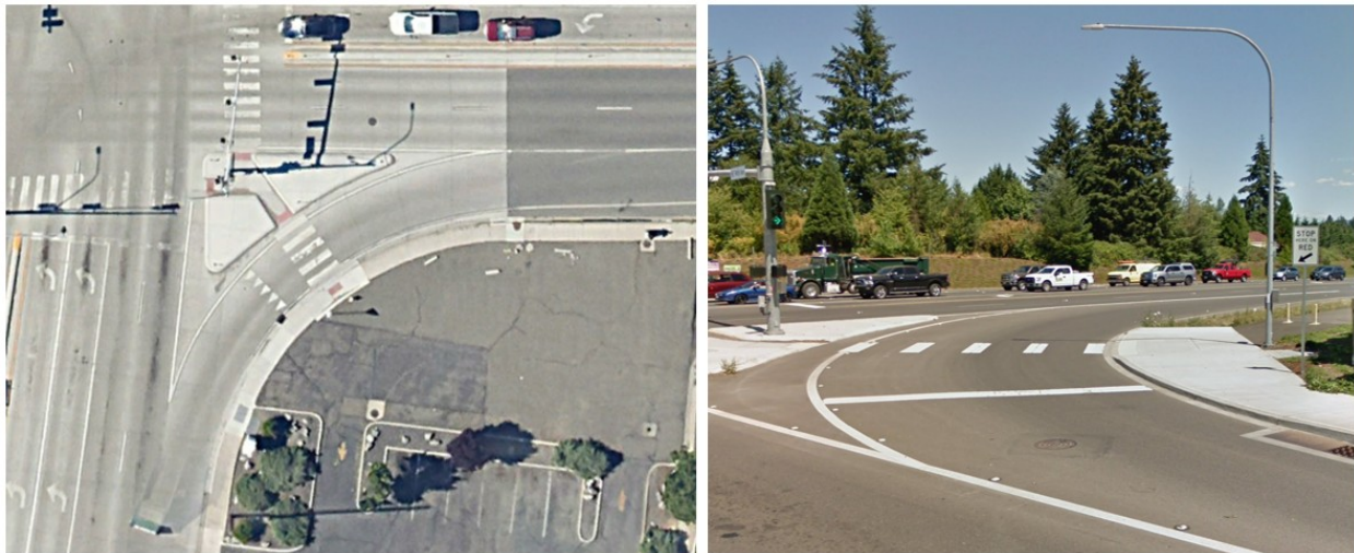
Figure 12. Examples of center-perpendicular crosswalk placement at CRTs [3].
