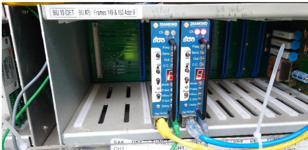
Figure 3.3. I-Loop Duo cards from the retired SMART Signal system at MN-55 site in Golden Valley.
