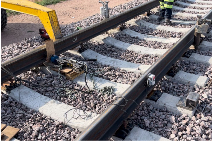
Figure 3: Photograph showing the operation of a single-tie push test experiment conducted by MxV Rail, Pueblo, CO
