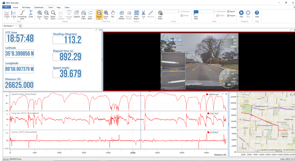
Figure 3-7: The interface of the VBOX software to visualize different attributes of the test run.
