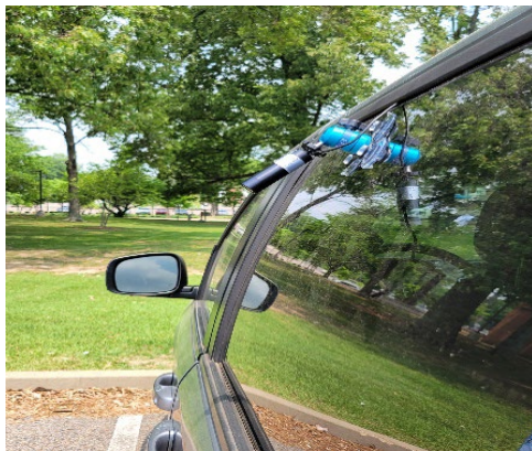
Figure 3-4: Camera installed on the left side.
