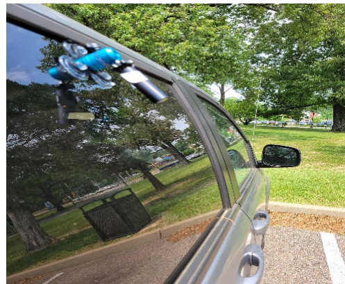
Figure 3-5 Camera installed on the right side.
