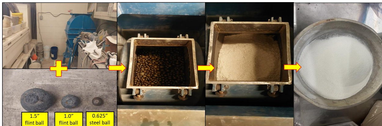
Figure 7. Ball mill machine and resulting ESP
