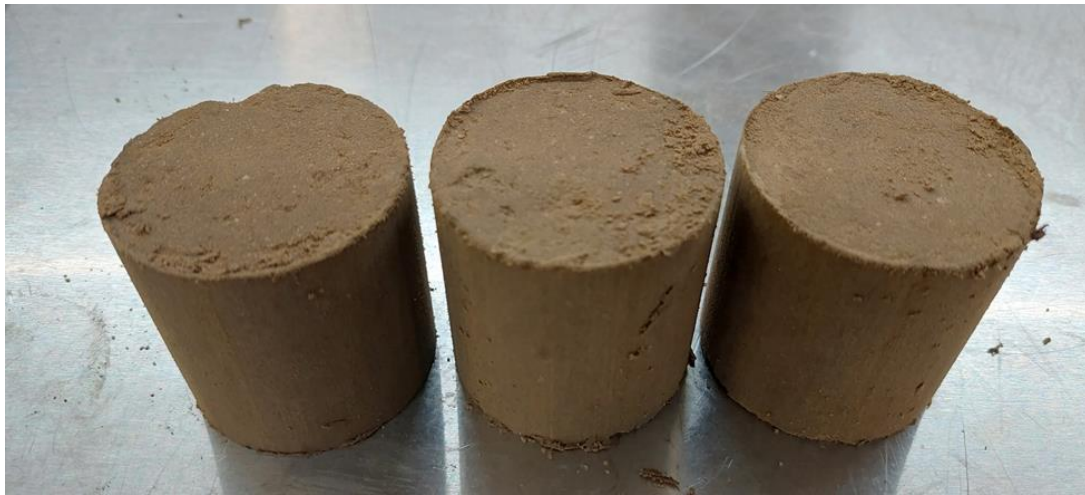
Figure 12. ESP-treated 2 in. by 2 in. soil specimens
