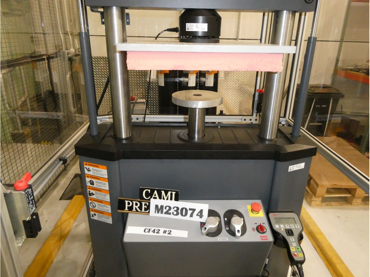
Figure C.1: ASTM D 3574 Type B test (IFD)
