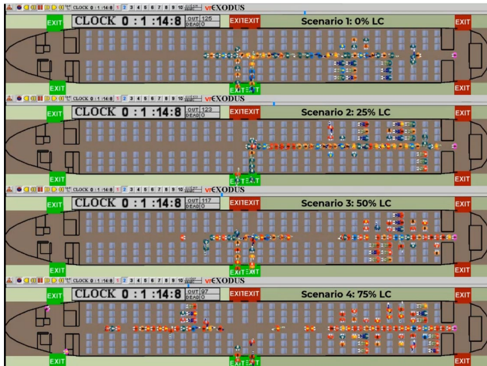
Figure 56: The predicted passenger distribution for the four scenarios (first image is Scenario 1) at 74 s into the simulations producing the median TET and demonstrating gap formation.
