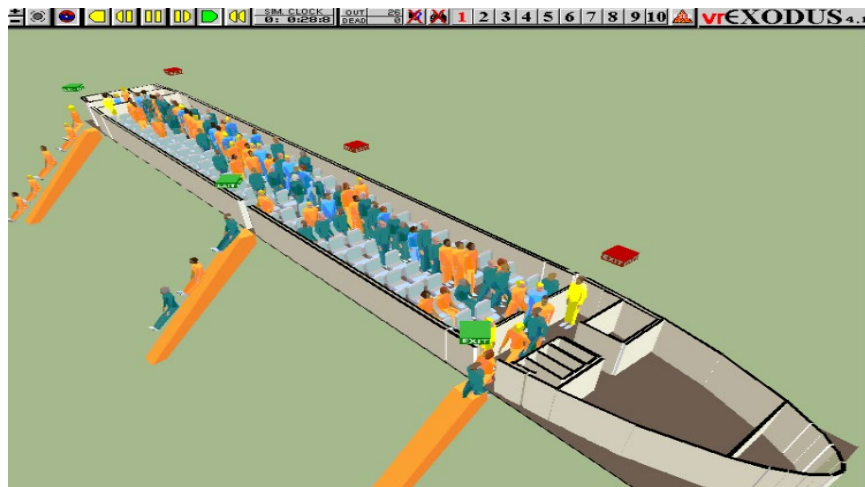
Figure 59: airEXODUS evacuation simulation depicted in the vrEXODUS software.
