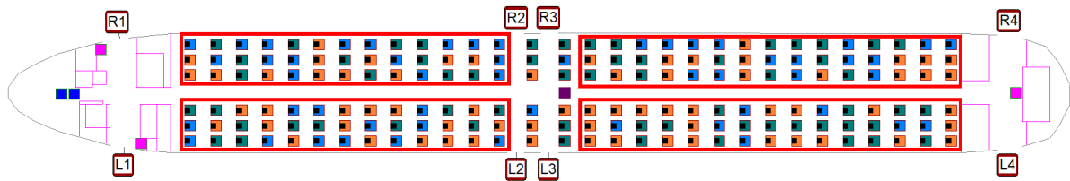
Figure 19: Luggage collector's zone consisting of four seat block regions covering the entire complement of seats, except for those seats that have aisles in front of them and lead to exits (i.e., between the L2/L3 and R2/R3 exits).
