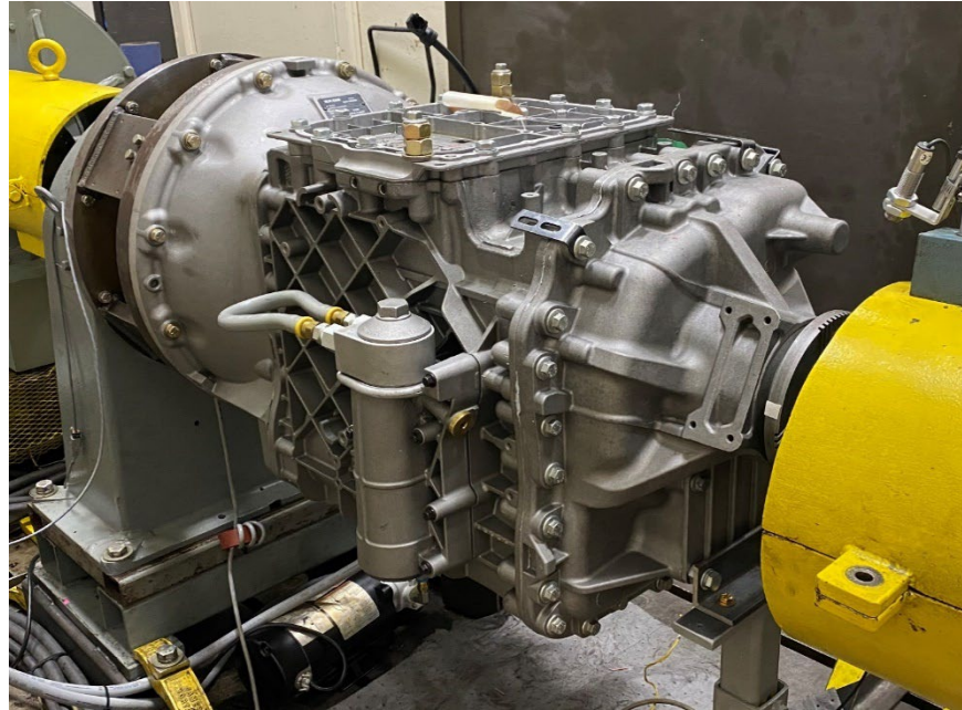
Figure 3. Volvo I-Shift transmission installed on the test stand
