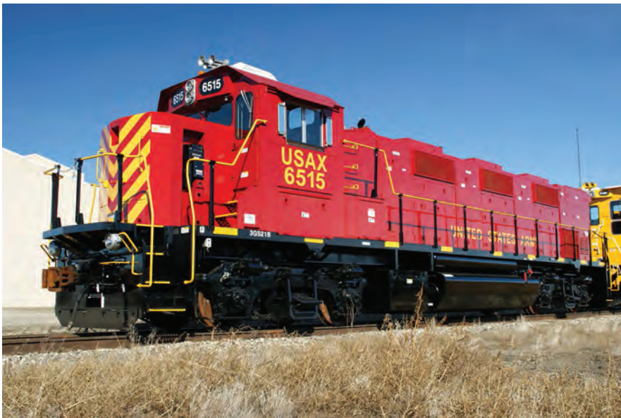
USAX 6515 is a three-engine 2,100-horsepower GenSet Road-switcher locomotive built to meet the requirements at Fort Liberty in North Carolina. This U.S. Army locomotive will be used to transport wheeled and tracked vehicles and other equipment maintained at this location. Source: U.S. DOT Volpe Center
