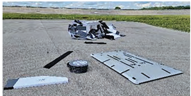
These images show the strikable vehicle soft test target and robotic platform. The target replicates real-world vehicle characteristics and dynamics and is placed on the robotic platform. It is built with foam and vinyl pieces to replicate physical vehicle characteristics but is made to withstand higher vehicle impact speeds (by breaking apart). The top right picture shows the vehicle broken down next to the vehicle platform. Source: U.S. DOT Volpe Center
