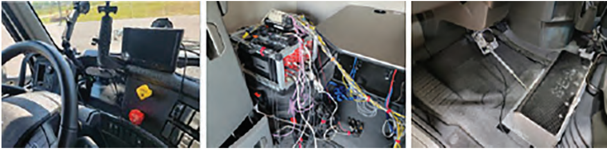
The vehicle interior instrumentation (left to right) to collect warning and braking activation times from the vehicle dashboard; collect test data about the vehicle and its surroundings; safely and accurately repeat throttle and brake conditions. Source: U.S. DOT Volpe Center
