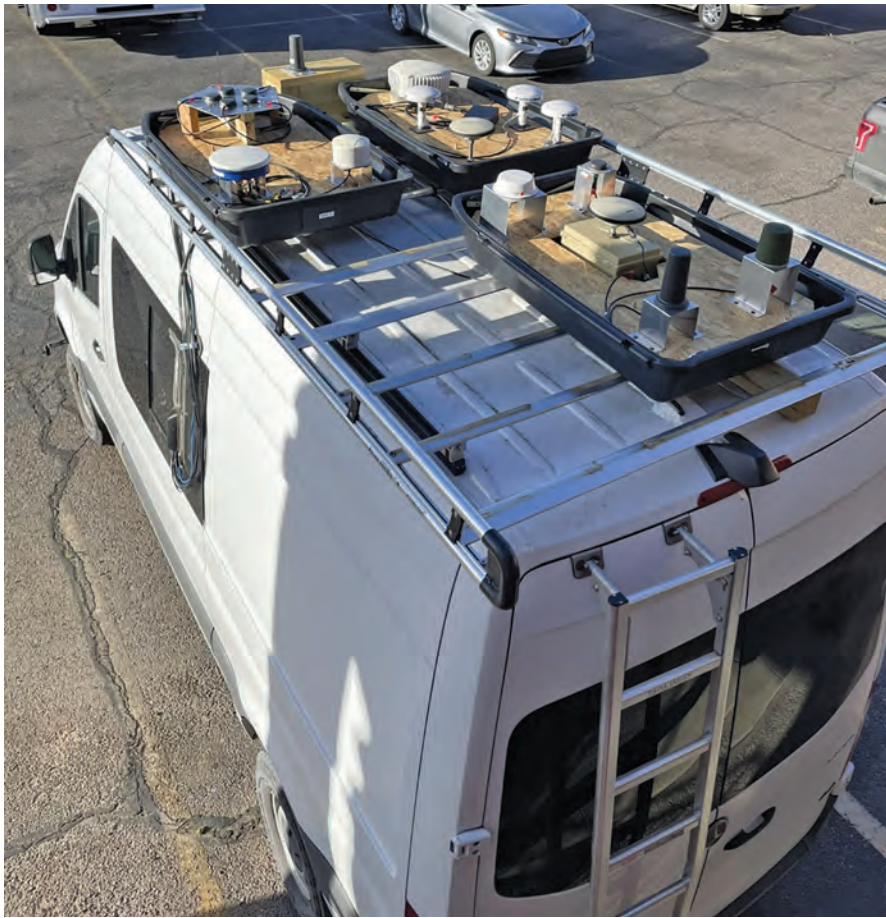
Antenna configuration on top of the U.S. DOT Volpe Center's Sprinter van prior to deployment. Source: U.S. DOT Volpe Center
