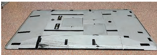
These images show the strikable vehicle soft test target and robotic platform. The target replicates real-world vehicle characteristics and dynamics and is placed on the robotic platform. It is built with foam and vinyl pieces to replicate physical vehicle characteristics but is made to withstand higher vehicle impact speeds (by breaking apart). The top right picture shows the vehicle broken down next to the vehicle platform. Source: U.S. DOT Volpe Center
