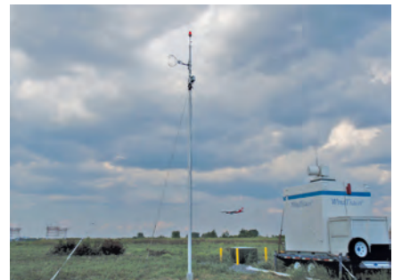
Measurement equipment used by U.S. DOT Volpe Center engineers to collect the data needed to support a wide range of wake turbulence analyses. Source: U.S. DOT Volpe Center
