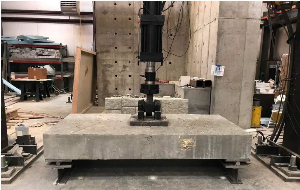
Figure 3.24 Failure load test setup
