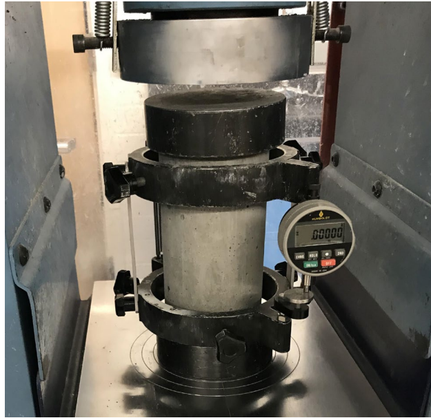
Figure 3.9 concrete Young's modulus test of cylinder
