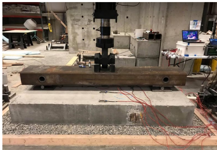
Figure 3.19 Cyclic loading test setup
