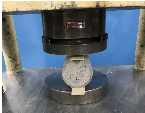
Figure 3.8 concrete split tensile strength test of cylinder
