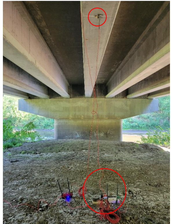
(b) Displacement transducer connected to bottom flange
