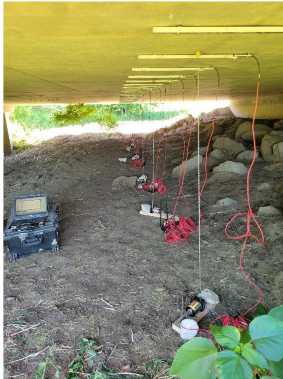
Figure 9. Strain gauges and displacement transducers on Bridge 9233.9S002
