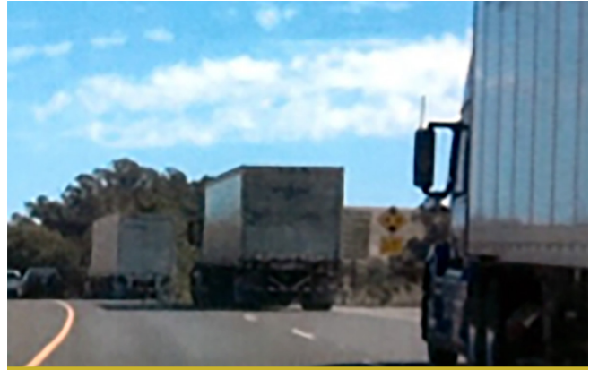
© University of California, Berkeley. Three Class-8 trucks equipped with CACC during field test.
