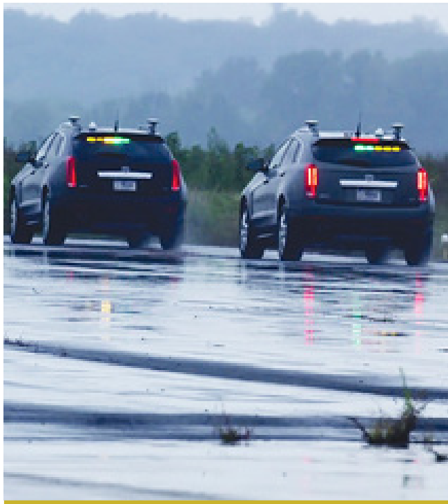
© Leidos. FHWA test vehicles simulate a “platoon” of vehicles using CACC.
