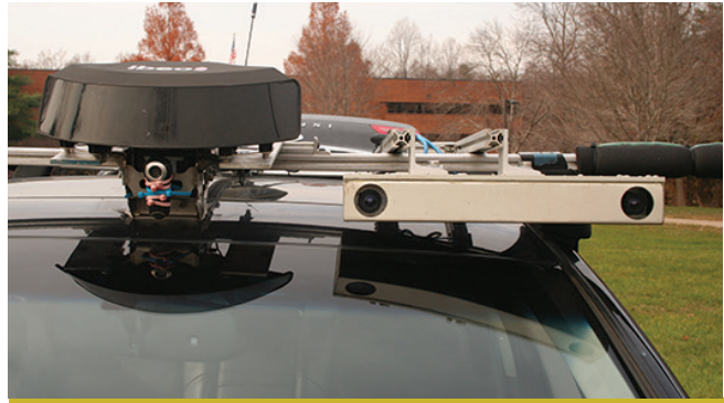
Source: FHWA. Camera and LIDAR equipment mounted on the roof of the test vehicle.
