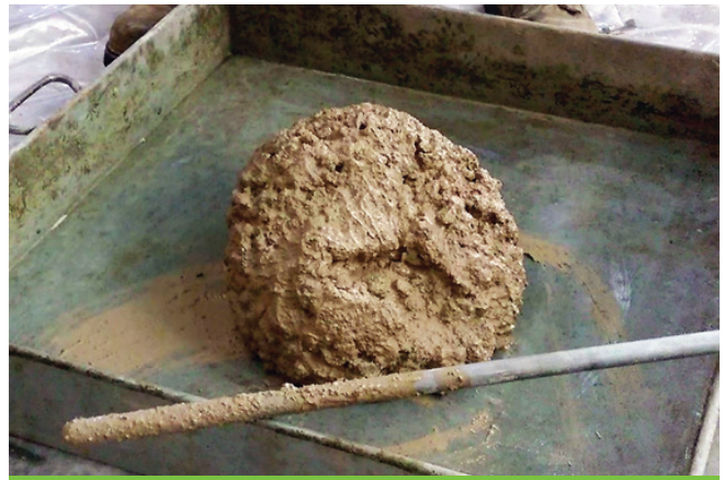
© College of Engineering, Georgia Institute of Technology. Concrete slump made of an alternative cementitious material (calcium sulfoaluminate).
