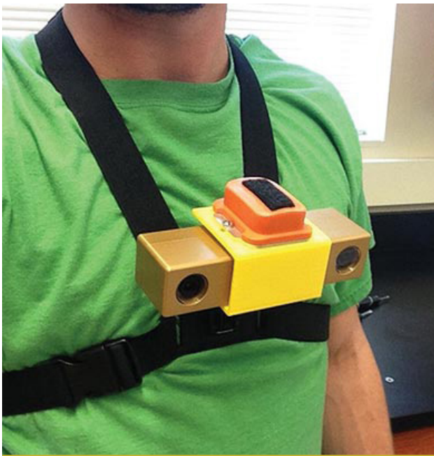
© Auburn University. A chest-mounted stereo camera and inertial measurement unit form part of Auburn University's pedestrian navigation system.
