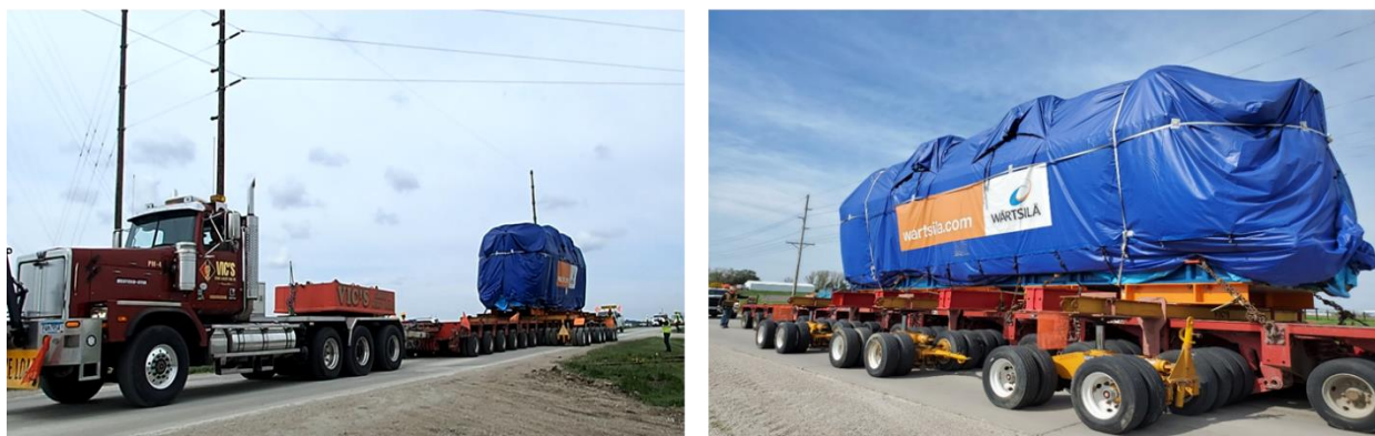
Figure 67. Body configuration of modular SHL with dollies that traveled road sections in Union County
