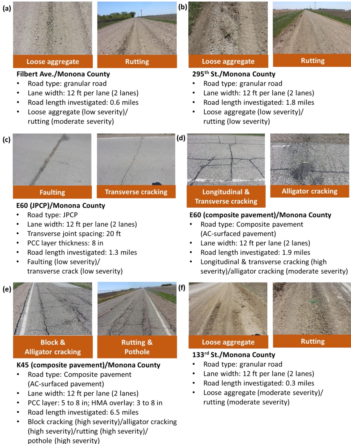
Figure 63. Summary of the forensic investigation results conducted in Monona County at (a) Filbert Avenue, (b) 295 th Street, (c) E60 (JPCP), (d) E60 (composite pavement), (e) K45, and (f) 133 rd Street
