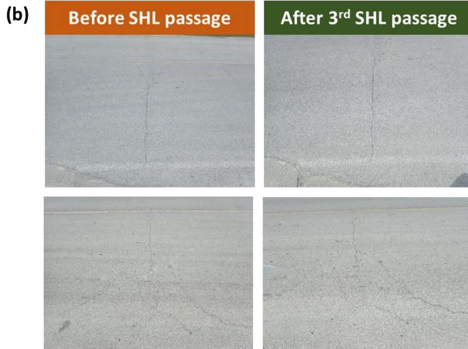
Figure 111. Comparison of distress severities before and after the third passage of the modular SHL over (a) Cherry Street and (b) Rea Road
