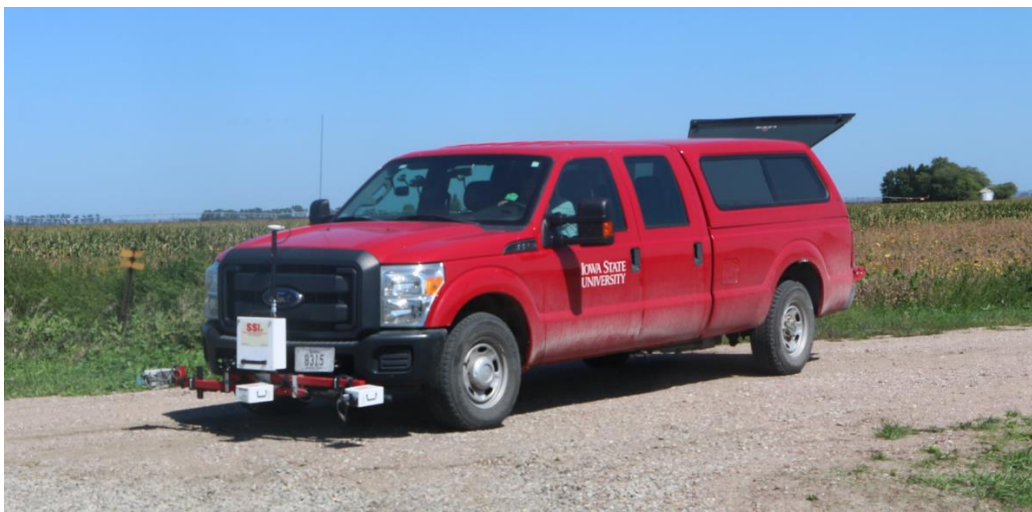
Figure 57. High-speed profiler used for IRI measurement
