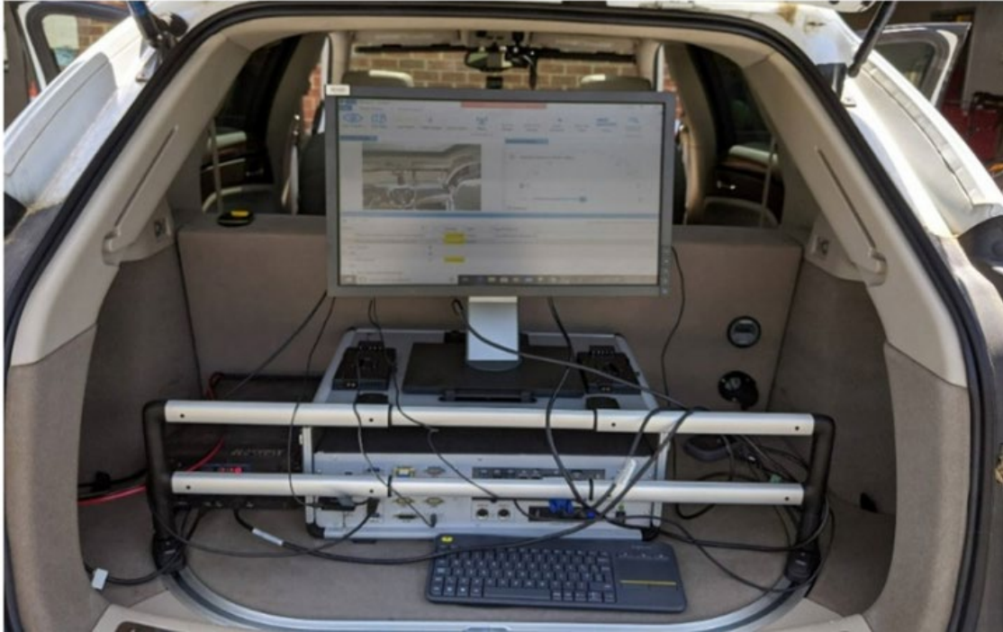
Figure 8. Photo. Data collection setup of the research vehicle.
