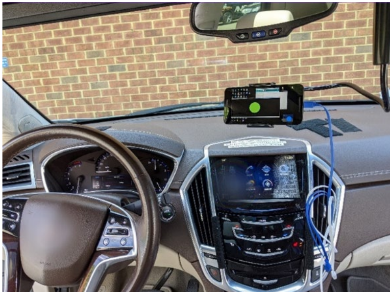
Figure 10. Photo. CDA message displayed on a smartphone mounted on the vehicle's dashboard.
